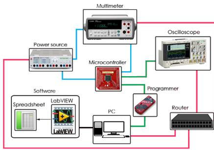
Fig. 3. A overview of the developed measurement system.
