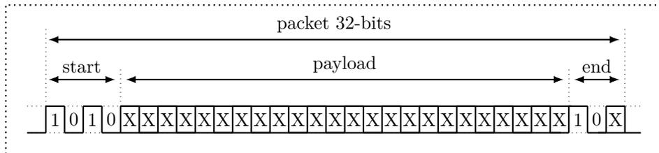
Figure 3.11: Measurement Packet Structure
