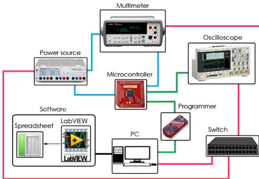
Fig. 1. Measurement setup overview
