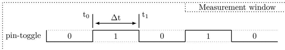
Figure 3.4: Measuring a Signal Duration on a Waveform
