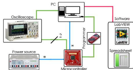
Fig. 1. An Overview of the Developed Measurement System [15].
