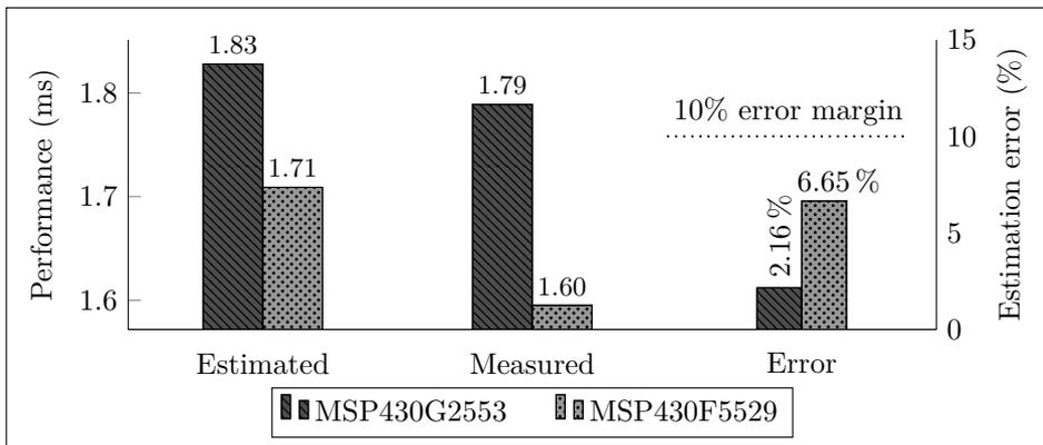
Figure 4.6: 16-bit MCU Performance Estimation of FIR Filter Benchmark
