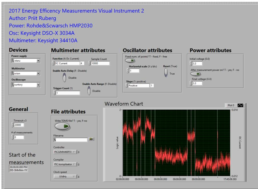
Figure 3.8: Front Panel View of LabVIEW for Energy Consumption Measurements
