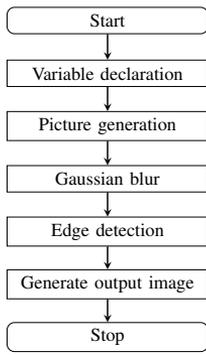
Fig. 3. Simplified image processing algorithm
