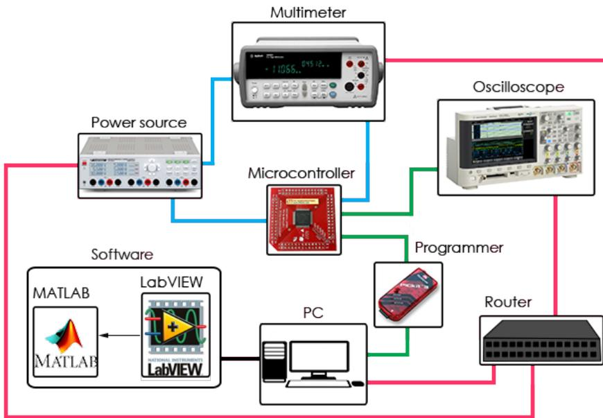
Figure 3.5: An Overview of the Automated Measurements System for Energy Estimation [67]
