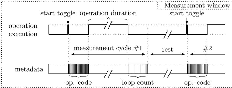
Figure 3.10: Measurement Window of 2-bit Protocol
