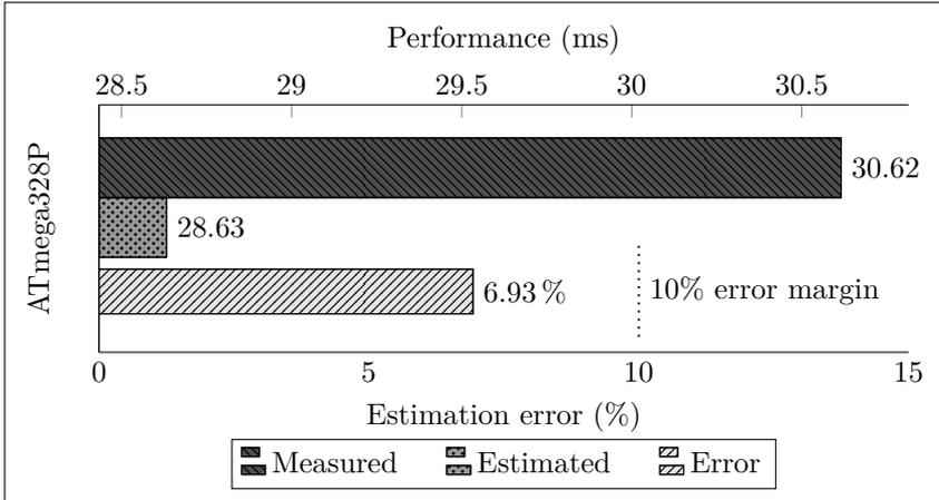
Figure 4.8: ATmega328P Performance Estimation of Image Processing Benchmark
