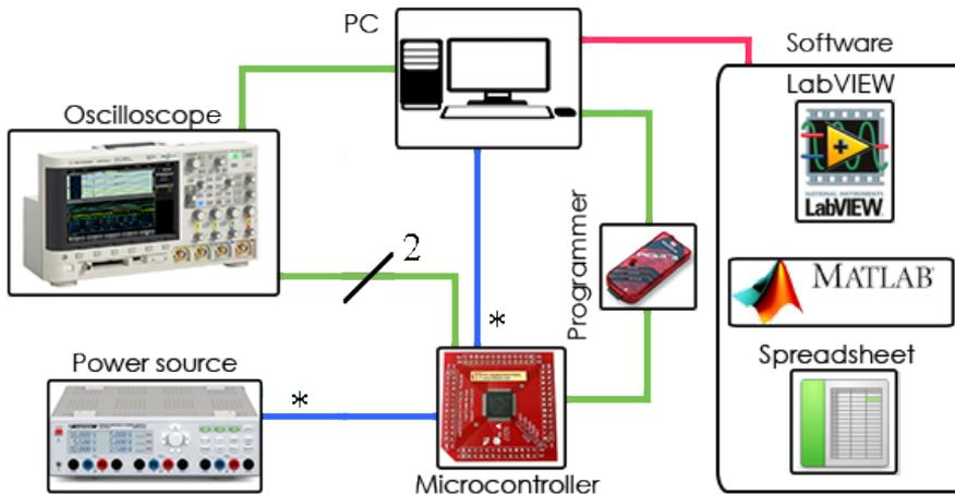
Figure 3.6: An Overview of the Automated Measurements System for Performance Estimation [69]
