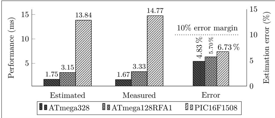
Figure 4.5: 8-bit MCU Performance Estimation of FIR Filter Benchmark
