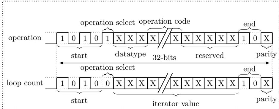
Figure 3.12: Packet Structure for "operation" and "loop count"
