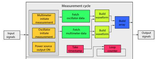
Fig. 5. A overview of the LabVIEW measurement cycle.
