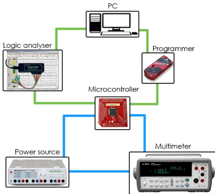
Figure 3.2: An Overview of the Initial Measurement System
