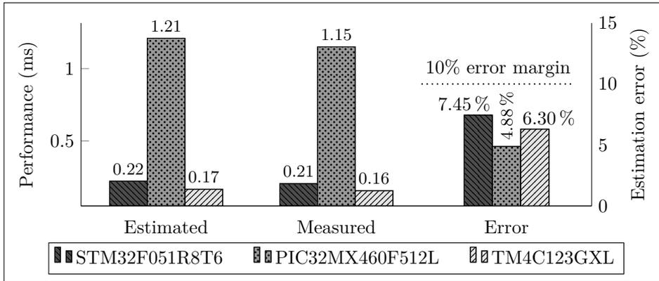
Figure 4.7: 32-bit MCU Performance Estimation of FIR Filter Benchmark
