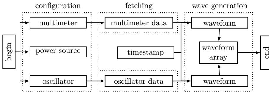
Figure 3.7: LabVIEW VI Block Diagram of Abstract Measurement Process
