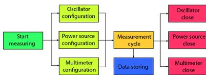
Fig. 4. A overview of the LabVIEW measurement system.
