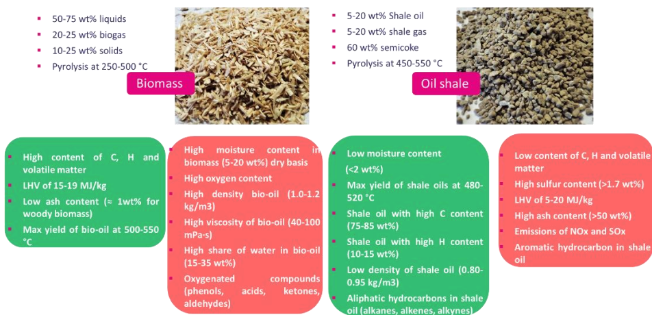
Figure 1. Yields of products and advantages (green) and disadvantages (red) of biomass and oil shale
