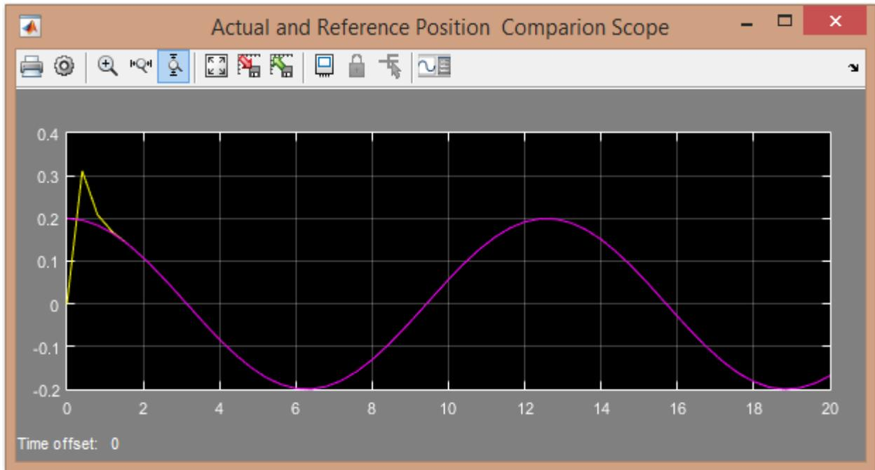
Figure 6.9: The robustness test curve with phase-shift of 90 degrees.
