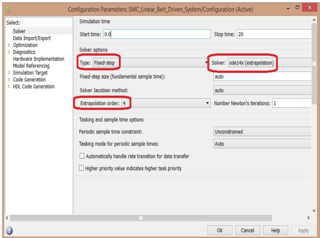
Figure 6.3: The solver settings needed to run the simulation
