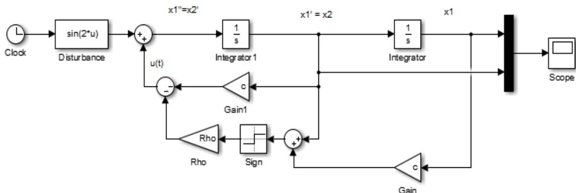
Figure 3.8: Simulink Model of the System with new control law
