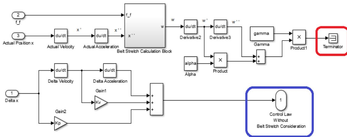
Figure 6.10: Removing the Belt Stretch Component from the Sliding Surface
