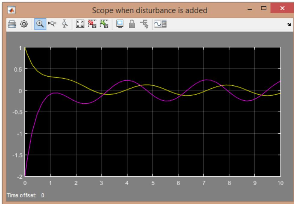
Figure 3.7: Convergence to a bounded domain when disturbance is added
