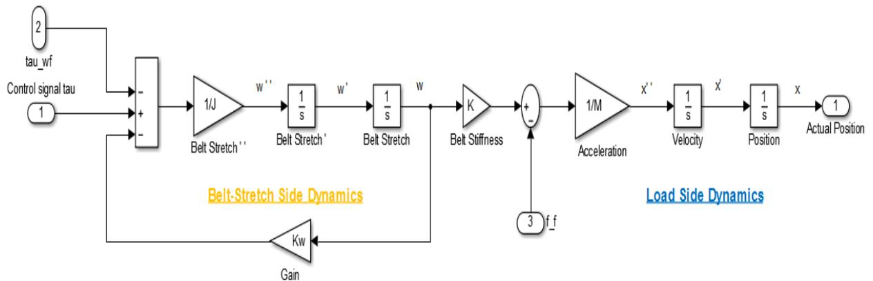
Figure 4.3: Block Scheme of Linear Belt-Driven System
