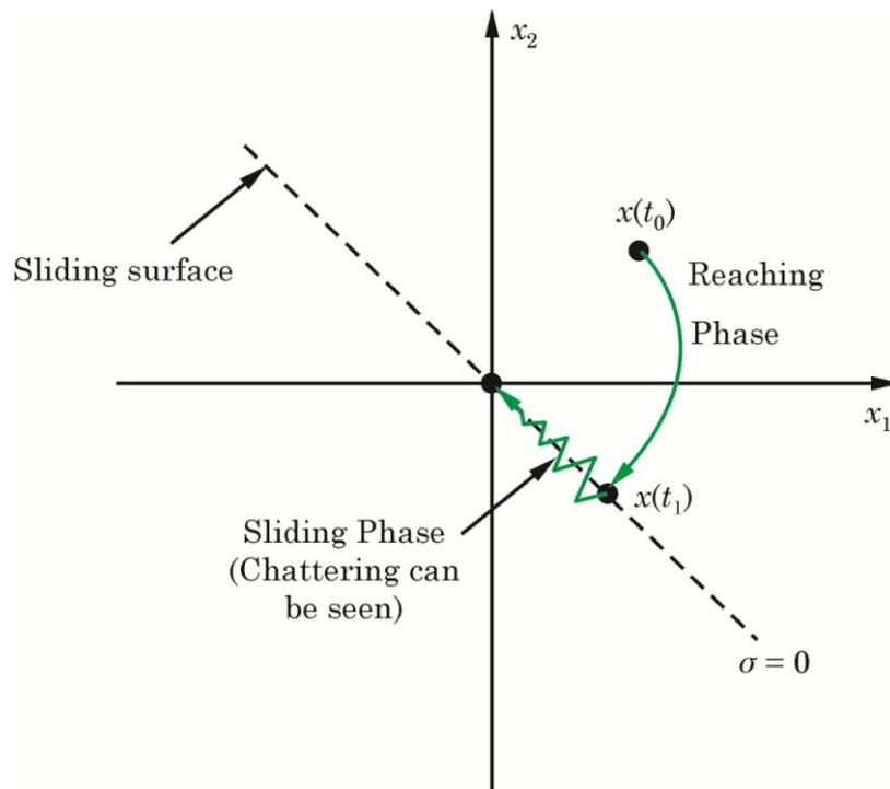
Figure 2.1: Reaching phase and Sliding phase
