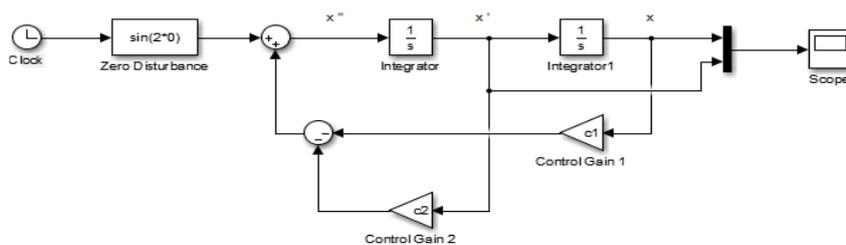
Figure 3.4: Simulink Model of the system when the disturbance is not considered
