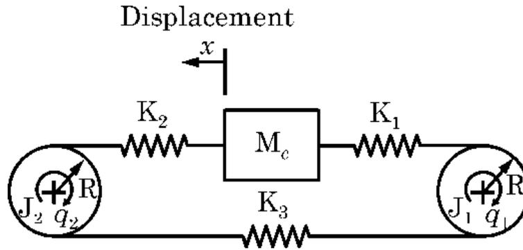
Figure 4.2: The Equivalent Spring-Mass System
