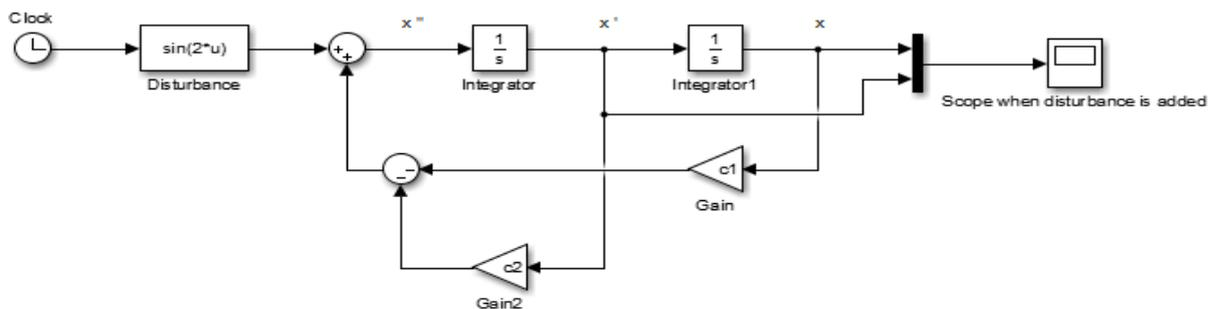
Figure 3.6: Simulink Model of the system when the disturbance is present
