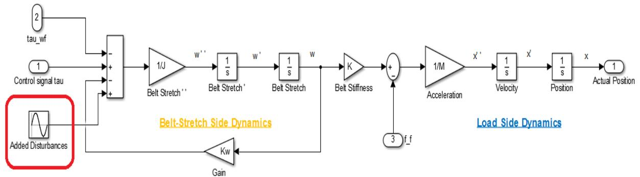
Figure 6.2: The Addition of Disturbances to the System
