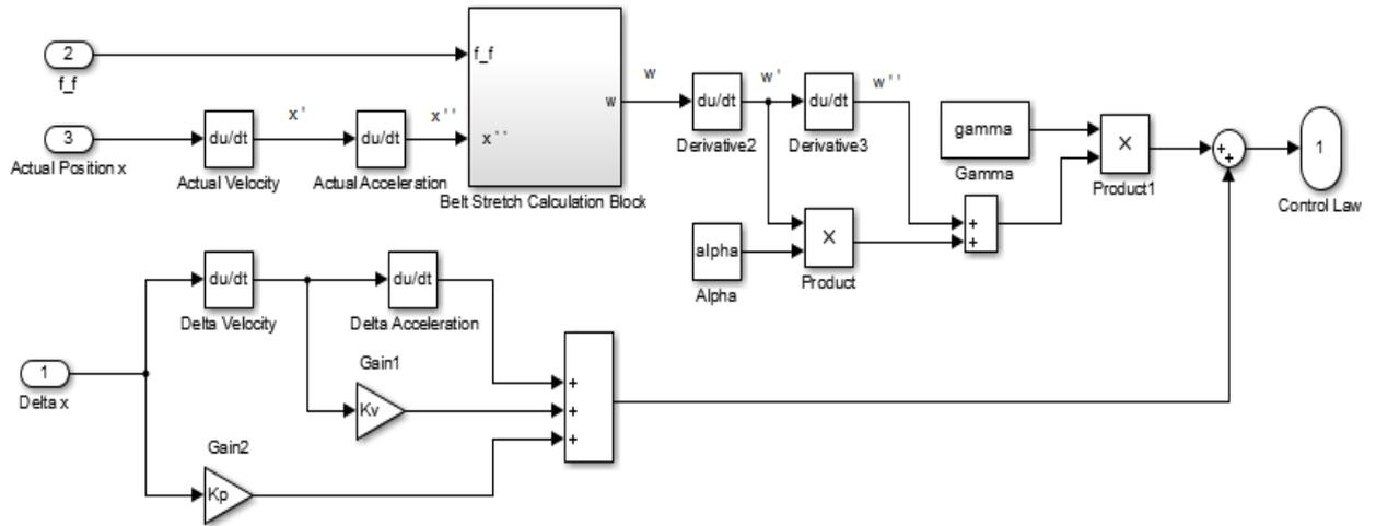
Figure 5.1: Control Law Deriving Procedure including the Belt-Stretch
