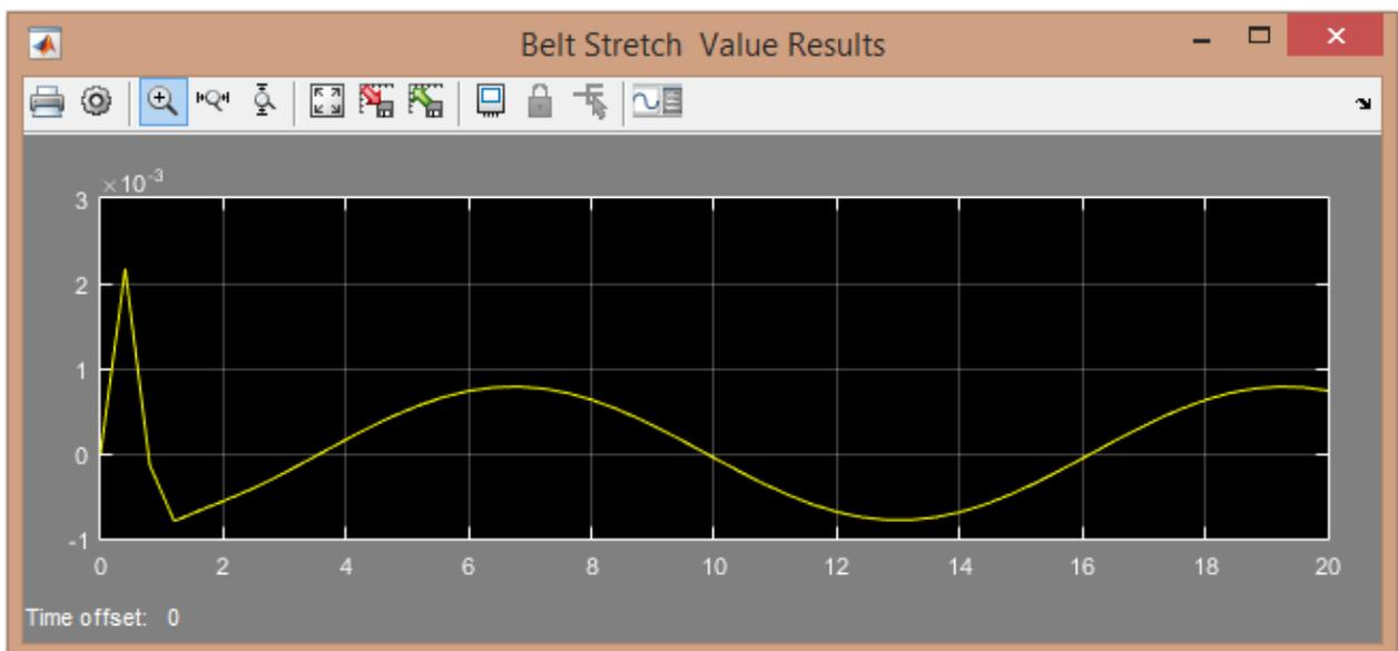
Figure 6.11: Belt Stretch Simulation Curve without Belt-Stretch Derivatives in Sliding Surface Design
