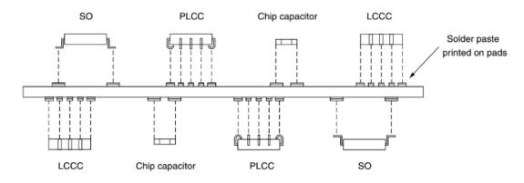
Figure 2.1 Schematic of type I surface mount boards [3]
