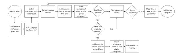
Figure 3.4 Kitting and preparation process
