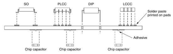
Figure 1.12 Schematic of type II surface mount boards
