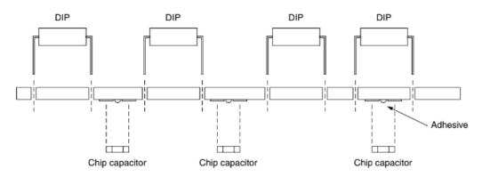
Figure 2.2 Schematic of type III surface mount boards [3]
