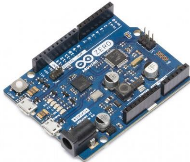
Figure 2.3 Arduino Zero board [7]
