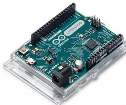
Figure 2.2 Arduino Leonardo board [7].
