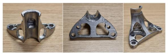
Figure 4.8 Guidance block near engine for wire bypass. Author's photos
