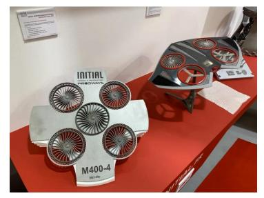
Figure 3.15 3D printed propellers at the Paris Air Show 2019 [31]
