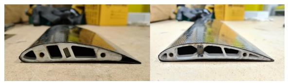
Figure 4.9 3D printed structures inside formula car wings. Author's photos
