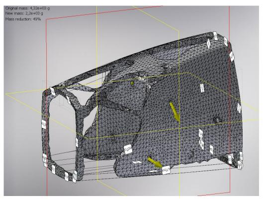
Figure 5.6 Topology optimization results, isometric view
