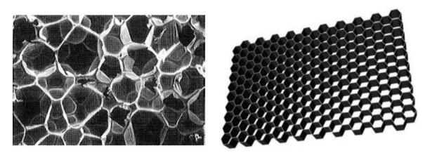
Figure 3.5 Different types of structures. On the left: foam, on the right: honeycomb [18]
