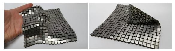
Figure 3.23 NASA 3D printed metal fabric [43]
