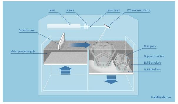
Figure 3.3 SLM principle [13]
