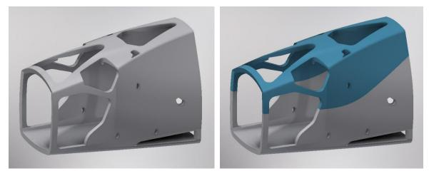
Figure 5.9 New model base on the left and divided model on the right
