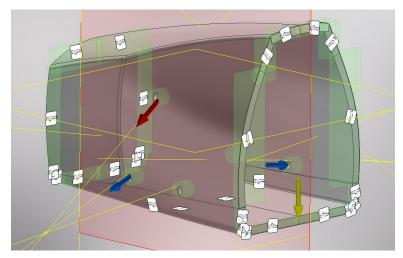
Figure 5.4 Isometric view of formula body part with forces and preserved areas
