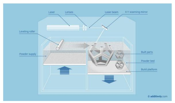
Figure 3.4 SLS printer [16]
