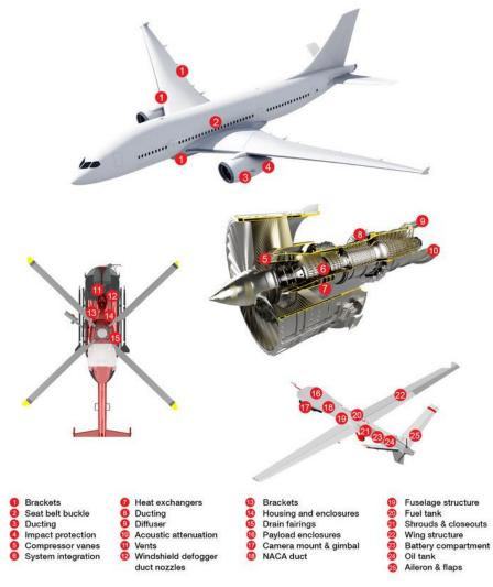
Figure 3.14 Aerospace AM applications [30]
