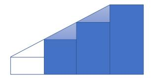
Figure 6.1 Idea of transition part between aluminium honeycomb and 3D printed structure
