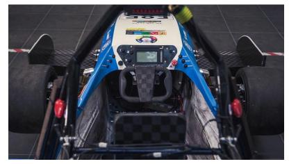
Figure 4.12 The steering wheel and inside of the formula student car [47]
