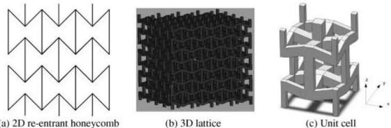
(a) 2D re-entrant honeycomb (b) 3D lattice Figure 3.6 Re-entrant honeycomb auxetic structure [19]
