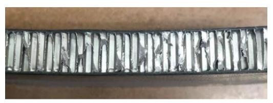
Figure 4.3 Cross-section of car body. Credit: Kaarel Haavajõe
