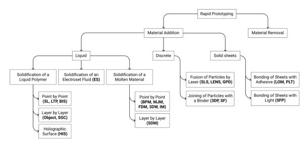
Figure 3.2 AM classification based on raw material state. (Source: [6]. Reproduced from Additive manufacturing: fundamentals and advancements)
