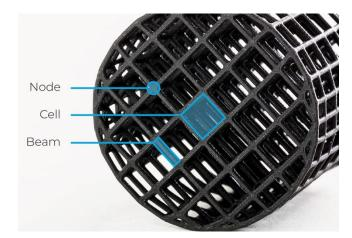
Figure 3.10 Lattice structure node, cell, beam [24]
