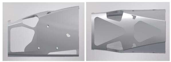
Figure 5.8 New model base generated through topology optimization
