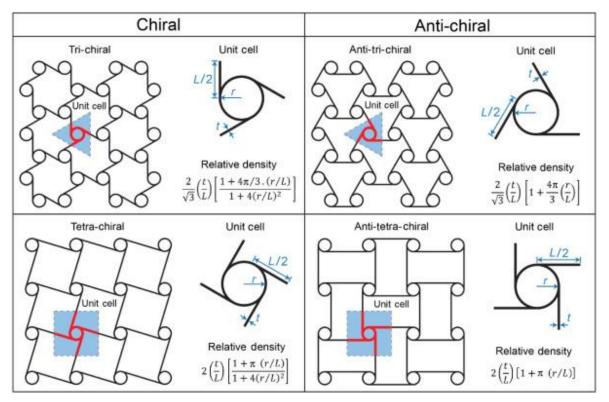
Figure 3.7 Schematic of the structure and unit cell for chiral and anti-chiral honeycombs [20]
