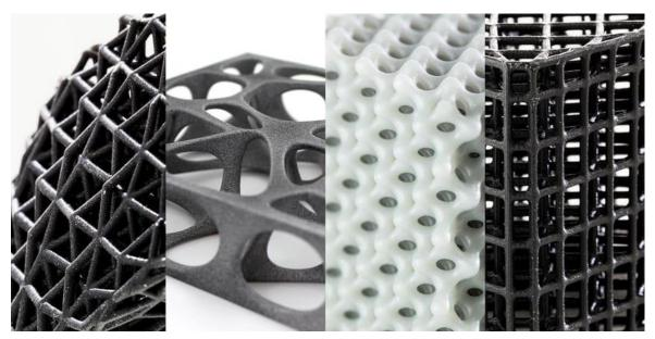
Figure 3.9 Lattice structures [24]
