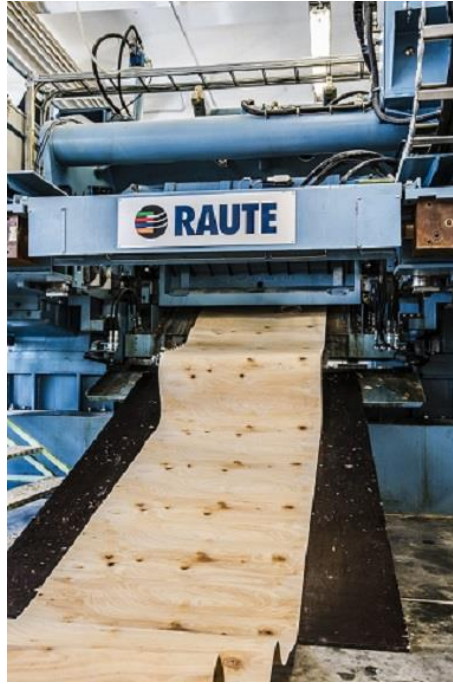
Figure 2.1 Raute veneer peeling machine [38]
