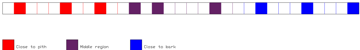
Figure 2.3 Selection of veneer sheets for testing (Image is schematic and does not represent constant order of selection. Sheet were selected after visually good surface quality and with fulfilling a need to select 3 random sheets from regions closer to bark, 3 from regions closer to pith and 3 from regions between)
