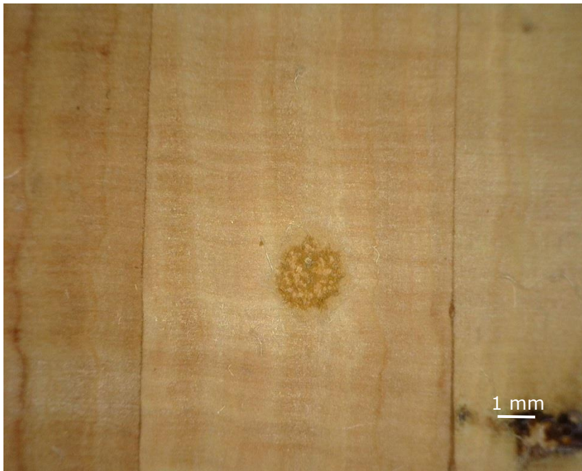
Figure A10.8 The first sample of cork material after 100 rubs seen through a microscope
