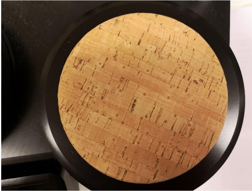
Figure A10.7 The first sample of cork material after 100 rubs
