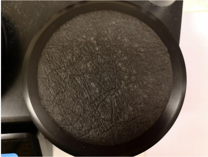
Figure A10.3 The first sample of Piñatex® material after 1000 rubs
