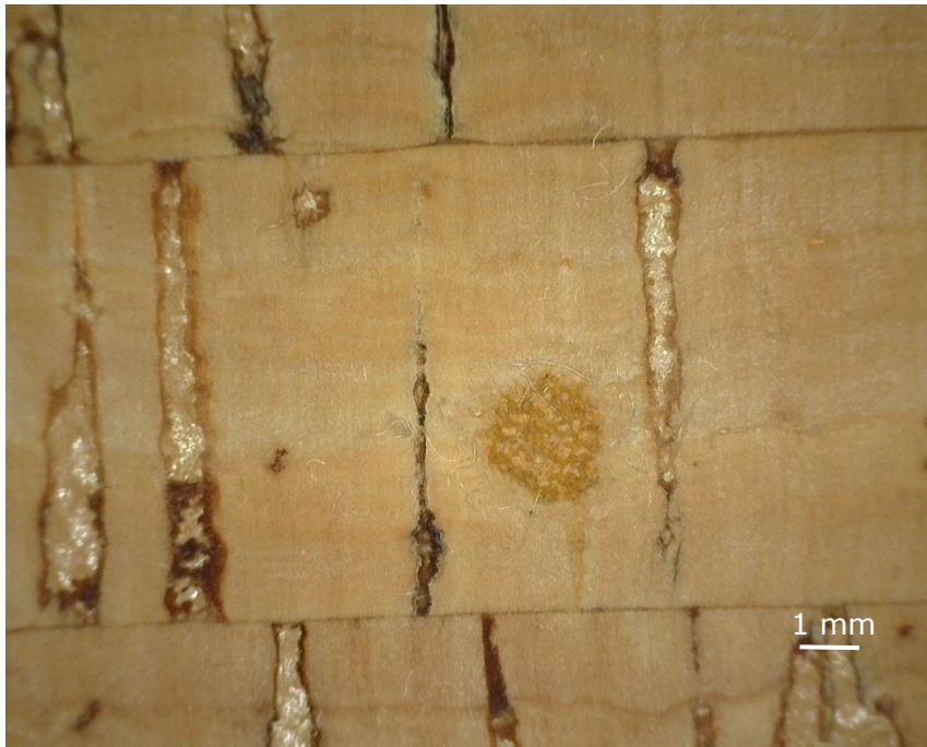
Figure A10.11 The second sample of cork material after 100 rubs seen through a microscope
