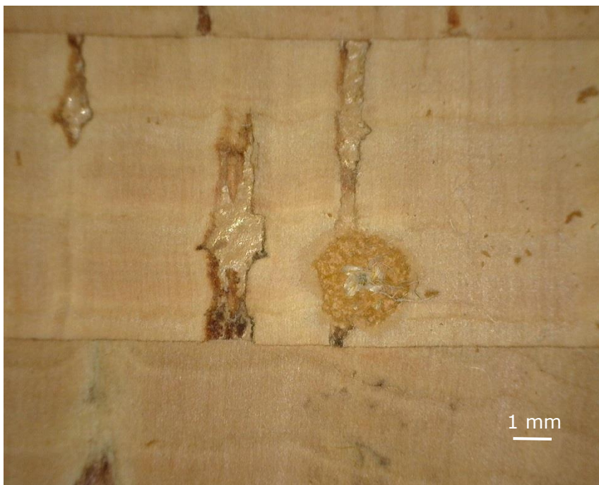
Figure A10.10 The first sample of cork material after 200 rubs seen through a microscope
