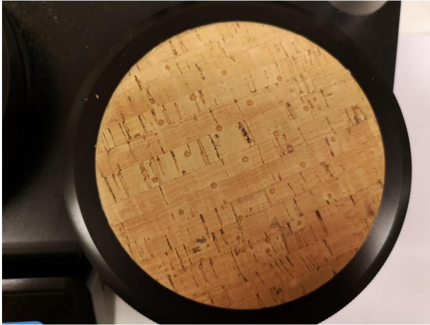
Figure A10.9 The first sample of cork material after 200 rubs
