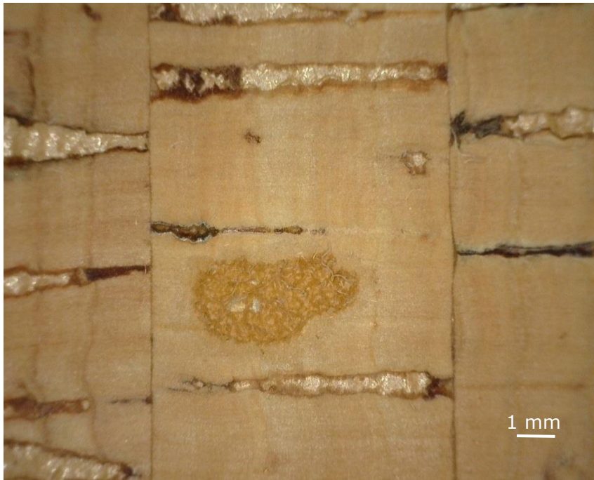
Figure A10.13 The second sample of cork material after 400 rubs seen through a microscope
