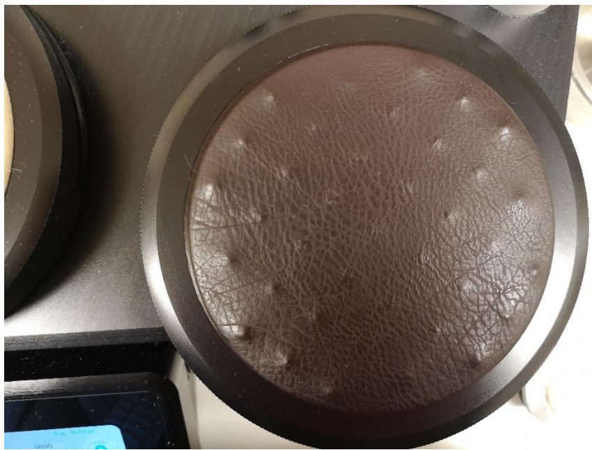
Figure A10.22 The first sample of PU covered fabric after 100 rubs
