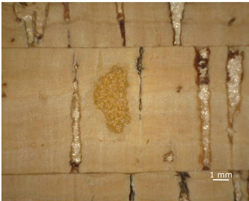
Figure A10.12 The second sample of cork material after 300 rubs seen through a microscope
