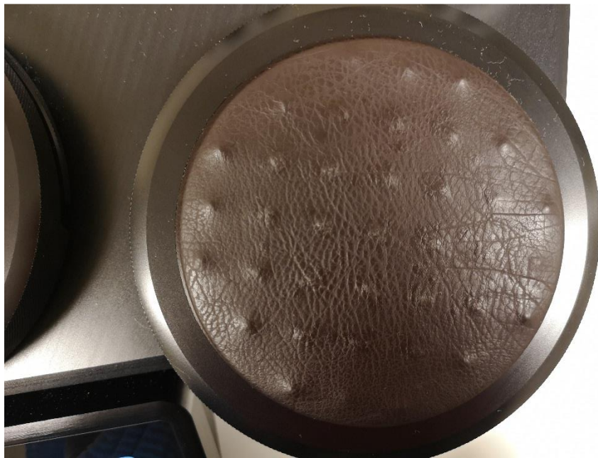
Figure A10.24 The first sample of PU covered fabric after 900 rubs
