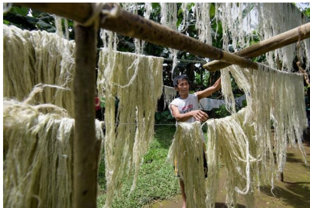
Figure 4.1.3 The fibres are then hung to dry before they are turned into a non-woven textile. [48]
