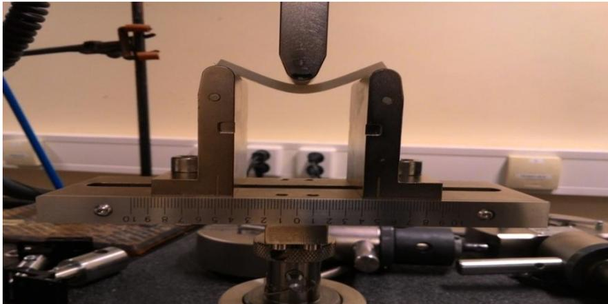
Figure 17. Three Point Load Bending Machine
