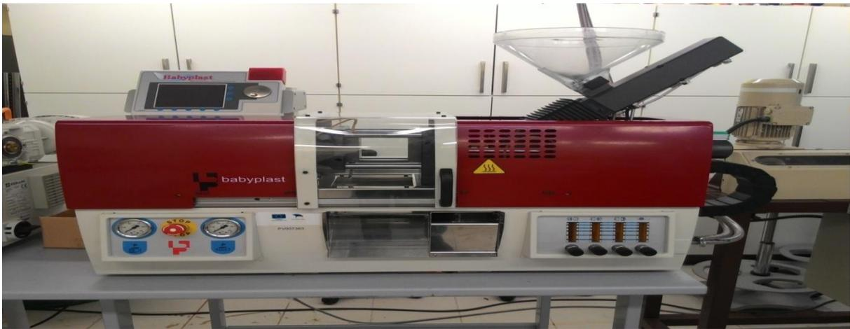
Figure 13. Babyplast 610P injection molding machine
