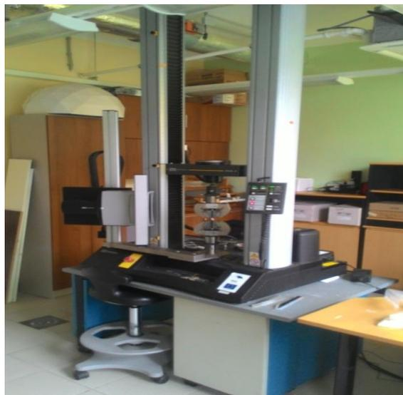
Figure 15. Universal Testing Machine (UTM) (Instron 5866)
