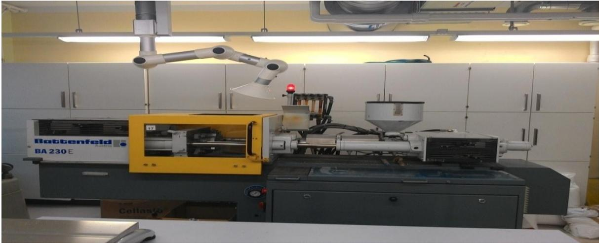
Figure 12. Injection Molding Machine (Battenfeld BA230E)
