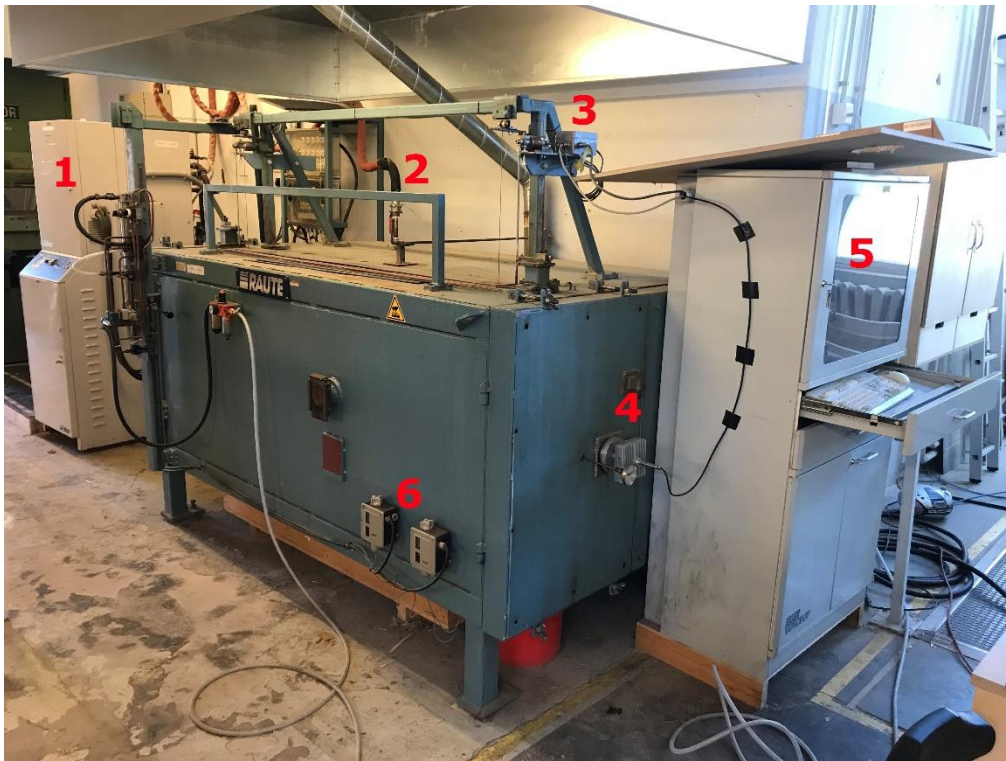
Figure 2.8. RAUTE Veneer dryer in Laboratory of Wood Technology
