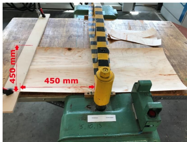
Figure 2.7. Veneer sizing with guillotine PM82
