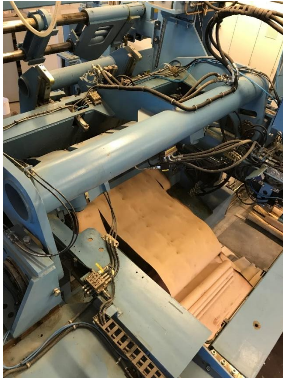
Figure 2.5. Veneer peeling with RAUTE lathe
