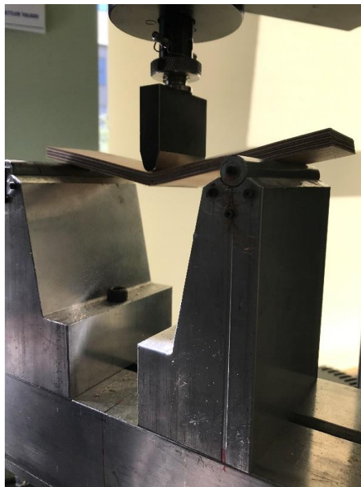
Figure 2.18. Plywood specimens bending strength test with Instron 5866
