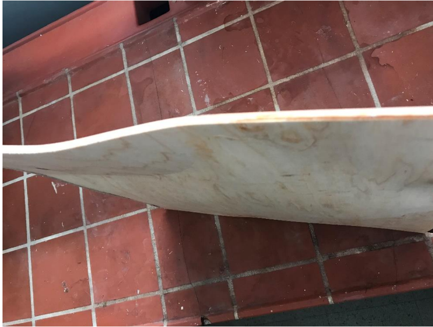
Figure 2.13. Example of buckled plywood panel after pressing
