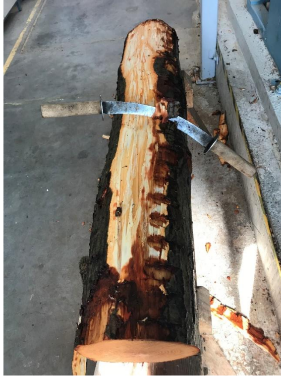
Figure 2.4. Debarking process with cutting knife
