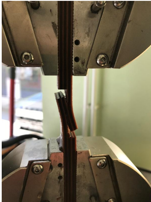
Figure 2.17. Shear strength specimen testing with Instron 5866
