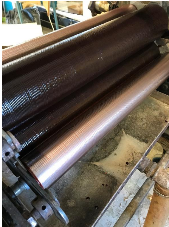
Figure 2.10. Black Brothers roller gluing machine filled with adhesive
