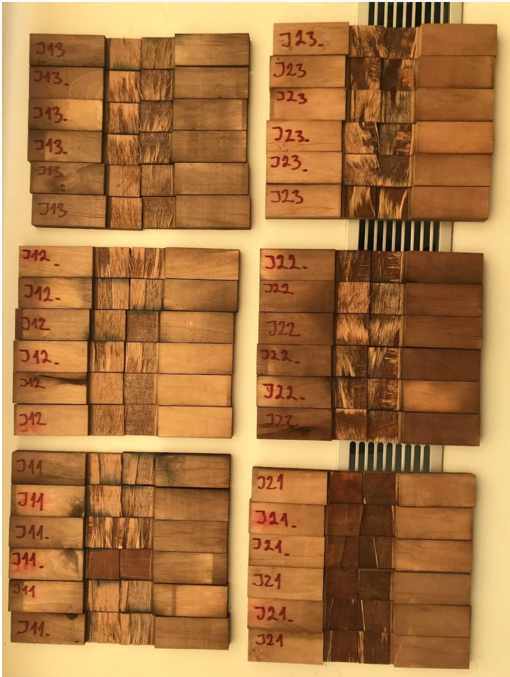
Figure A 1.2. Grey alder shear strength specimens
