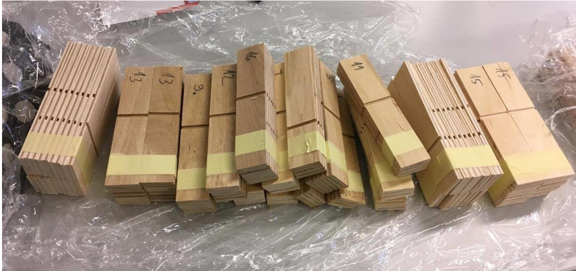
Figure 2.4. Specimens for shear strength testing
