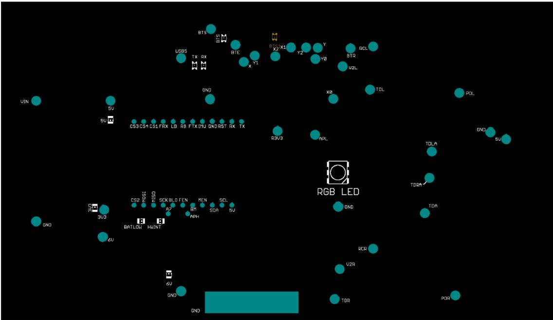
Figure 24. Test pads and LEDs (Eagle rendering). Test pads (green), LEDs on the top layer (white) and LEDs on the bottom layer (orange).
