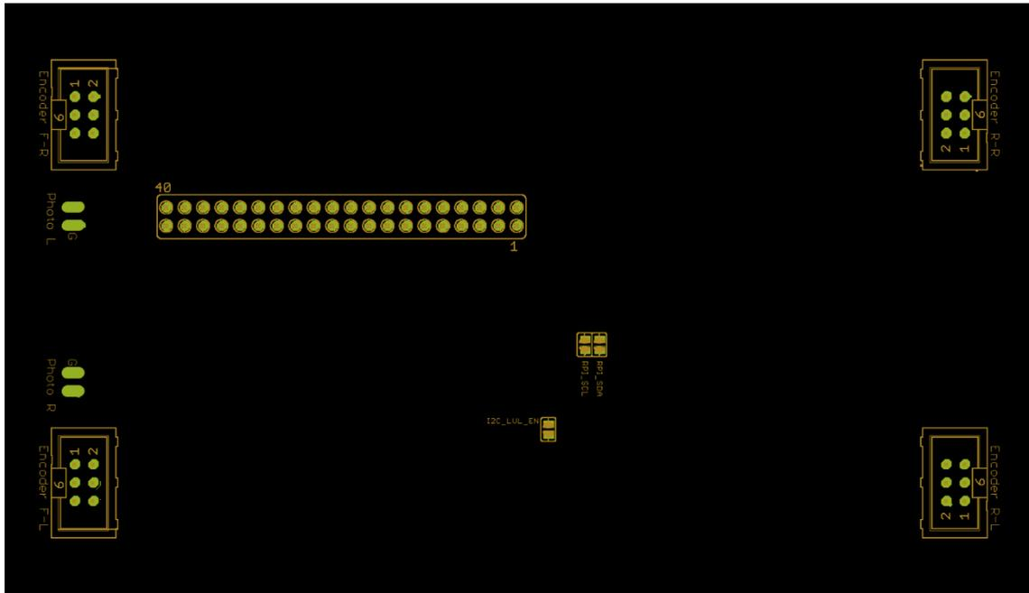
Figure 26. Connectors and jumpers on the bottom layer (Eagle rendering).
