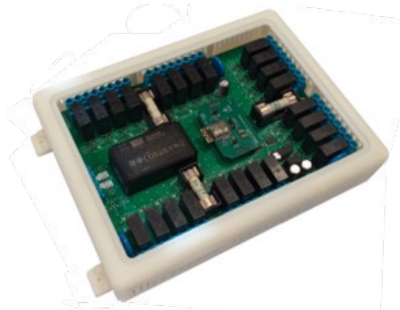
Figure 2.8 Demand simulation controller board.
