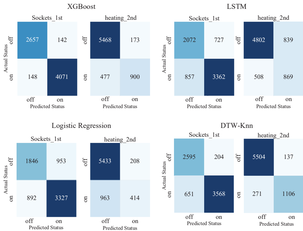
Figure 9. Confusion matrices obtained for specific threshold value.
