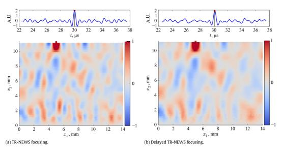
**Fig. 11.** Extent of the material affected by high amplitude ( $A_{max} > 1$ ) focused wave in case of TR-NEWS focusing and delayed TR-NEWS focusing for  $\Delta \tau = 0.25 \ \mu$ s,  $a_i = \{1, 1\}$ . Unnormalized results are shown with focusing maximum amplitude  $A_{max} > 2.0$ . Additional video files are available in the supplementary materials (see Appendix A).
