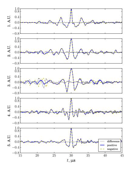
Figure 10 – PI nonlinearity depending on the receiving transducer position near 1 mm defect (A.U. - amplitude units). Figure from Publication V.
