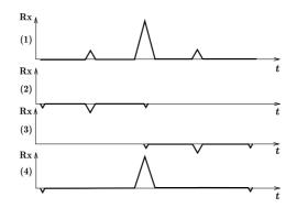
**Fig. 6.** Scheme of the side lobe reduction using delayed TR-NEWS: (1) initial  $y_{TR}$  focusing with side lobes (Eq. (5)); (2) and (3) scaled and shifted focusing for eliminating side lobes; (4) resulting  $y_{dTR}$  from adding together signals (1)-(3) has reduced side lobes but slightly reduced main peak.
