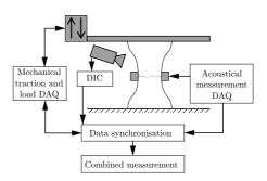
Figure 13 – Acoustomechanical test setup using mechanical and acoustic measurements (DAQ–Data Acquisition, DIC–Digital Image Correlation). Figure from Publication IV.
