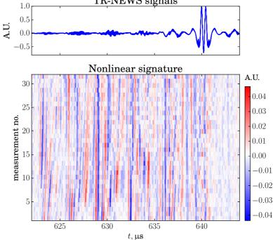
Figure 16 – Top: 32 delayed TR-NEWS signals with two generated peaks. Bottom: the difference between the predicted and measured delayed TR-NEWS wave interaction (nonlinearity). Time  $t = 640 \mu s$  is the initial TR-NEWS focusing time.
