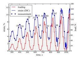
Figure 5: Strain and load at a selection of measurement points
