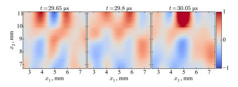
Figure 8 – Wave interaction caused by delayed TR-NEWS with a single delay focusing. Coordinates are denoted by  $x_1$  and  $x_2$ , focusing takes place at  $t = 30 \,\mu\text{s}$ . Figure from Publication II.
