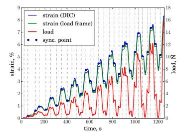
Figure 14 – Synchronised mechanical data from skin sample extension, with TR-NEWS synchronisation points
