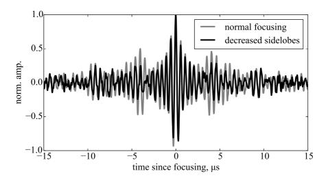
Figure 6 – Delayed TR-NEWS focusing experiment with a CFRP sample. By superpositioning two time-delayed and scaled copies of the focused pulse on the sidelobes, the relative size of the sidelobes can be decreased. Figure from Publication II.
