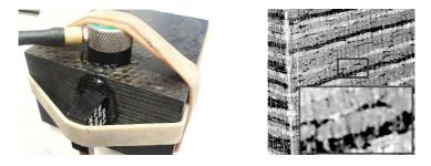
Fig. 1. Carbon Fibre Reinforced Polymer (CFRP) block (left) and its structure (right). This test configuration was chosen arbitrarily in order to verify the practical feasibility of the method in an NDT test.
