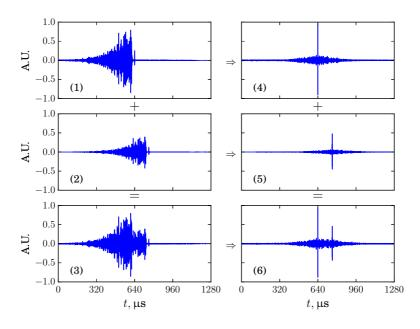
Figure 2 – Delayed TR-NEWS steps. Left column: superposition of crosscorrelations. Right column: superposition of focused waves. (1) Cross-correlation (Eq. (3)); (2) delayed and scaled cross-correlation; (3) linear superposition of two cross-correlations (Eq. (5)), which becomes the new excitation; (4) focusing (Eq. (4)); (5) delayed and scaled focusing; (6) linear superposition of the two focusing peaks (Eq. (6)).
