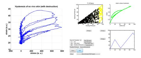
Figure 3: Skin PM space for memory analysis extracted from hysteretic strainstress measurements conducted on ex vivo porcine skin. Optimization of the strainstress curve induces a PM space with 600 hysterons distributed along a Guyer distribution[17]. This original result constitutes the first PM-space identification of viscoelastic and/or hysteretic properties of the skin under uniaxial loading.
