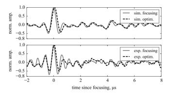
Fig. 10. Comparison of delayed TR-NEWS in simulation (upper subfigure) and experiment (lower subfigure) with 0.25 µs delay, comparing the widening of the pulse.
