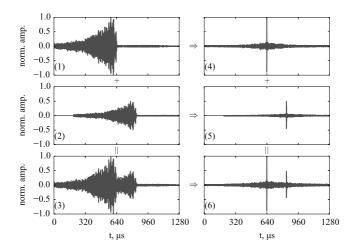
**Fig. 5.** Delayed TR-NEWS signal processing steps conducted in bi-layered aluminium, starting from the cross-correlation step (left column) and prediction of linear superposition of waves (right column): (1) cross-correlation (Eq. (4)); (2) delayed and scaled cross-correlation; (3) linear superposition of two cross-correlations which becomes the new excitation; (4) focusing (Eq. (5)); (5) delayed and scaled focusing; (6) Linear superposition of the two focusing peaks.
