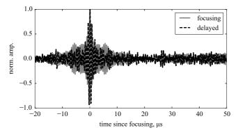
**Fig. 9.** Improvement of focusing in bi-layered aluminium due to delayed TR-NEWS experiment with delay  $\Delta \tau = 0.25 \,\mu s$  and  $a_i = \{1, 1\}$ .
