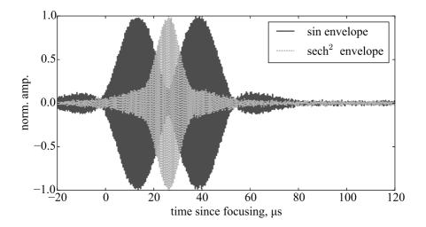
Figure 7 – Delayed TR-NEWS in CFRP for creating a specially shaped envelope at the focusing. Figure from Publication II.
