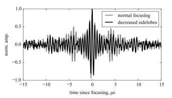
Fig. 16. Results of a delayed TR-NEWS focusing experiment with the CFRP sample: due to using of two time-delayed and scaled copies of the original signal the size of the side lobes can be reduced significantly compared to normal focusing.
