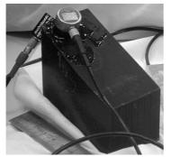
**Fig. 1.** Carbon Fibre Reinforced Polymer (CFRP) block of 144 layers tested with ultrasonic of NDT.
