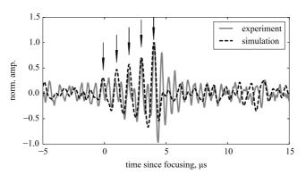
**Fig. 8.** Comparison of the delayed TR-NEWS CFRP physical experiment and simulation. The five peaks are delayed with intervals  $\Delta \tau = 1 \mu s$  and have relative amplitudes  $a_i = \{0.1, 0.2, 0.3, 0.4, 0.5\}$ .
