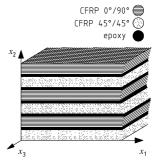
Fig. 3. Material model of the CFRP block.
