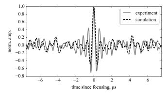
Fig. 7. TR-NEWS wave focusing in CFRP, comparison of the TR-NEWS simulation with the physical experiment.
