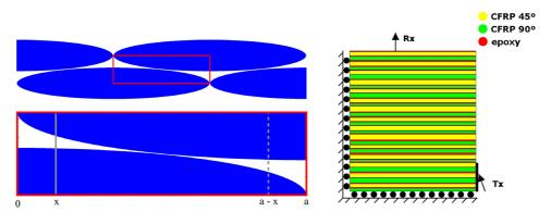
Fig. 2. The material consisting of elliptic yarns in tight packing (left) is modelled as a laminate with stochastic thicknesses of layers (right) due to different possible wave paths encountering different thicknesses of CFRP yarn and epoxy.
