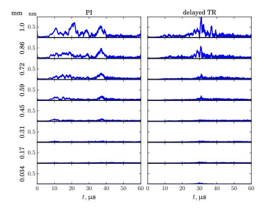
Figure 11 – Comparison of nonlinear signature envelopes in displacement  $u_2$  using PI and delayed TR-NEWS for defect size from 1 mm to 0.034 mm. Figure from Publication V.
