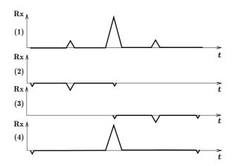
Figure 5 – Scheme of the sidelobe reduction using delayed TR-NEWS: (1) initial  $y_{\text{TR}}$  focusing with sidelobes (Eq. (4)); (2) and (3) scaled and shifted focusing for eliminating sidelobes; (4) resulting  $y_{\text{dTR}}$  of adding together signals (1)–(3) with reduced sidelobes and slightly reduced main peak. Figure from Publication II.
