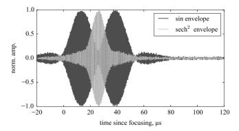
Fig. 15. Delayed TR-NEWS in CFRP for creating an envelope of special shape at the focusing.
