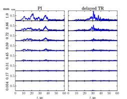
Figure 12: Comparison of the PI and delayed TR-NEWS nonlinearity measure envelopes (deformation  $u_2$  difference in nm) depending on the size of the defect (in mm)
