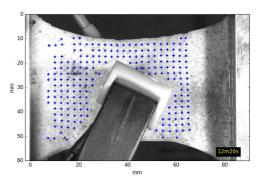
Figure 2: DIC frame with displacement markers added in post-processing. The extension is toward right (video available at [10]).
