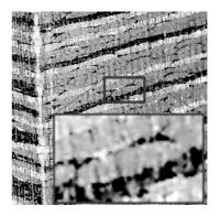
Figure 4 – Structure of the CFRP with the fabric yarns in tight packing and epoxy filling the voids. Figure from Publication II.
