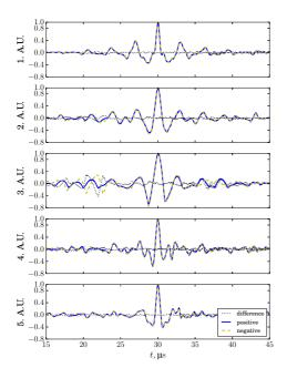
Figure 7: (Colour online) Normalized TR-NEWS focusing of damaged CFRP simulation with PI applied to detect nonlinearities as difference between negative and positive excitations
