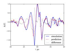
Figure 11: (Colour online) Delayed TR-NEWS nonlinearity measure between predicted and simulated values from position 3 on 1 mm damage with delayed peak amplitude  $a_i = 1$  and delay value  $\tau = 1$  µs (Eq. (2))
