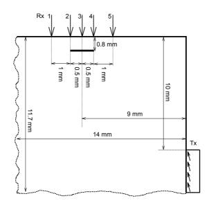
Figure 9 – Schematic of the simulation setup (not to scale) with the transmitting transducer (Tx) position on lower right, receiving transducer (Rx) positions (1-5) on top and the defect just below the Rx position. Figure from Publication V.
