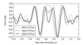
Fig. 14. Delayed TR-NEWS focusing manipulations in CFRP experiment with three different delay values, showing different moments of converging wave interaction at the focusing moment.
