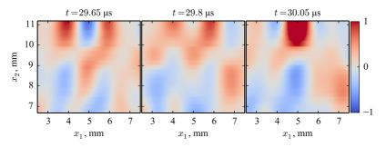
Fig. 13. Several separate waves arriving and interacting in CFRP simulation of the focusing.
