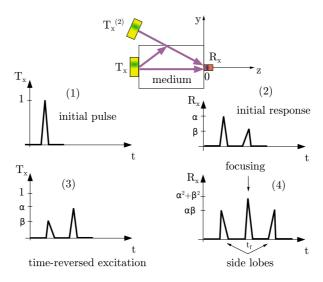
Figure 1 – TR-NEWS virtual transducer concept: (1) the initial broadband excitation  $T_x(t)$  propagates in a medium; (2) additional echoes from interfaces and scatterers as new virtual sources  $T_x^{(2)}$ ; (3) time reversal; (4) response  $y_{\text{TR}}(t)$  with a spatio-temporal focusing at z = 0; y = 0;  $t = t_f$  and symmetric sidelobes with respect to the focusing. Figure from [42].
