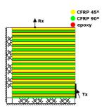
Figure 3: (Colour online) The laminate material model with layers of stochastic thicknesses and absorbing boundary conditions on bottom and left boundaries and four fixed degrees of freedom
