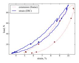
Figure 7: A single hysteresis loop in the test in the timespan from 550 s until 675 s, with round markers showing the synchronization points of TR-NEWS measurements
