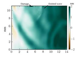
Figure 10: (Colour online) TR-NEWS focusing to pos. 3 at time  $t = 32.6 \ \mu s$ , showing displacement  $u_2$  wave emission coming from the damaged region. Video available at [27]
