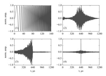
Fig. 4. Chirp-coded TR-NEWS signal processing steps in bi-layered aluminium experiment: (1) chirp excitation; (2) output recorded at Rx; (3) crosscorrelation between input and output; (4) focusing resulting from transmitting the time-reversed cross-correlation as a new ultrasonic input.
