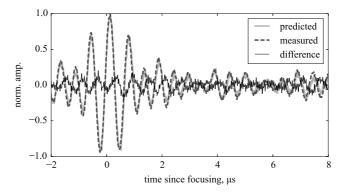
**Fig. 12.** Prediction from delayed TR-NEWS signal processing ( $\Delta \tau = 0.25 \,\mu$ s) versus the results from actual experiment in bi-layered aluminium sample.
