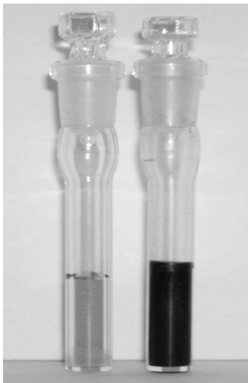
Picture 1. The performance of Estonian oil shale solvent swelling experiments. The left taste-tube corresponds to the beginning of the experiment when the oil shale sample is introduced into the tube. The right taste-tube corresponds to the swollen sample
