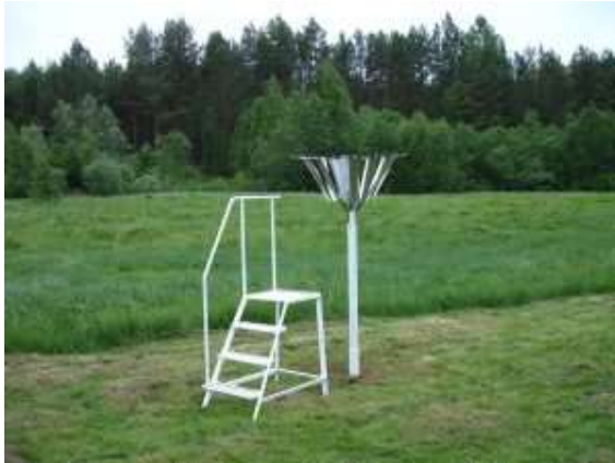
A Tretyakov precipitation gauge.
