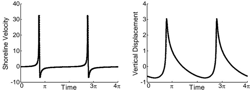
Fig. 2.5.5. Velocity and vertical displacement of the moving shoreline for a nonlinear deformed wave ( $s/s_0 = 10$ ) in non-dimensional variables; the breaking parameter  $Br = 0$  (dotted line),  $Br = 0.5$  (dashed line) and  $Br = 1$  (solid line)
