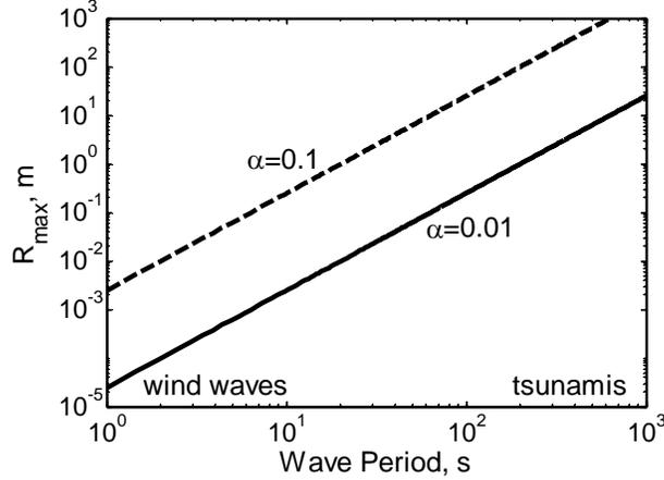
Fig. 2.3.1. The breaking criterion for long waves on a plane beach
