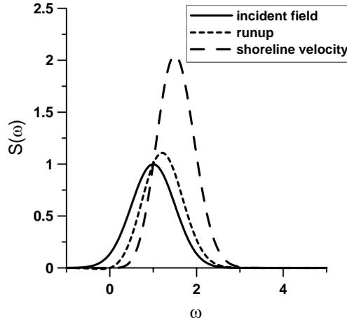
Fig. 3.3.1. Incident field, runup and shoreline velocity spectra for  $l = 0.5$
