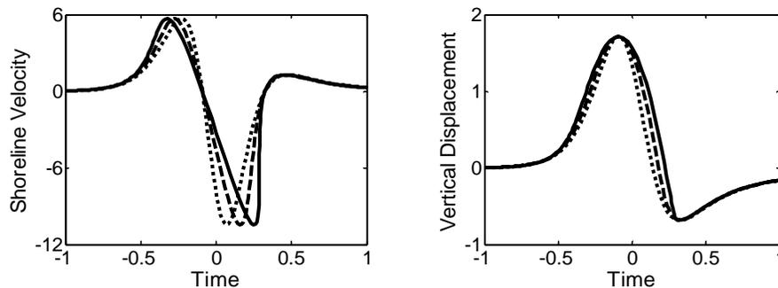
Fig. 2.4.4. Velocity and vertical displacement of the moving shoreline (dimensionless variables) for the incoming KdV soliton; the breaking parameter  $Br = 0$  (dotted line),  $Br = 0.5$  (dashed line) and  $Br = 1$  (solid line)
