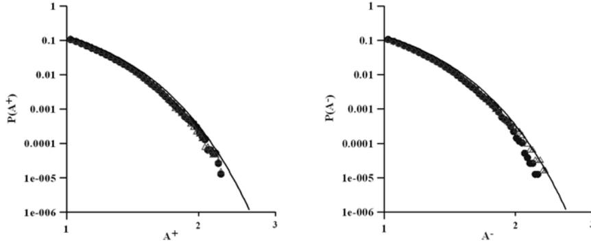
Fig. 3.4.1. Distribution functions of maximum positive (left) and negative (right) amplitudes for incident wave (triangles) and shoreline displacement (circles) with the incident wave spectrum width  $l = 0.7$ . The solid line corresponds to the Rayleigh distribution
