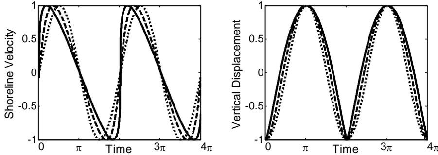
Fig. 2.3.2. Velocity and vertical displacement of the moving shoreline (dimensionless variables) when the sine wave approaches the coast for  $Br = 0.2$  (dotted line),  $Br = 0.5$  (dashed line) and  $Br = 1$  (solid line)
