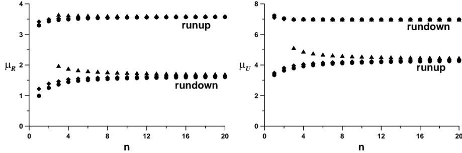
Fig. 2.4.2. Calculated form factors for the maximum runup ( $\mu_R^+$ ) and rundown ( $\mu_R^-$ ) heights and runup ( $\mu_U^+$ ) and rundown ( $\mu_U^-$ ) velocities for sine power pulses (triangles), soliton-like (diamonds) and Lorentz-like (circles) impulses
