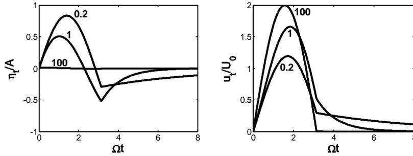
Fig. 1.5.4. The shape of the transmitted wave (left) and transmitted velocity (right) after the inflection point for various values of the parameter  $q$
