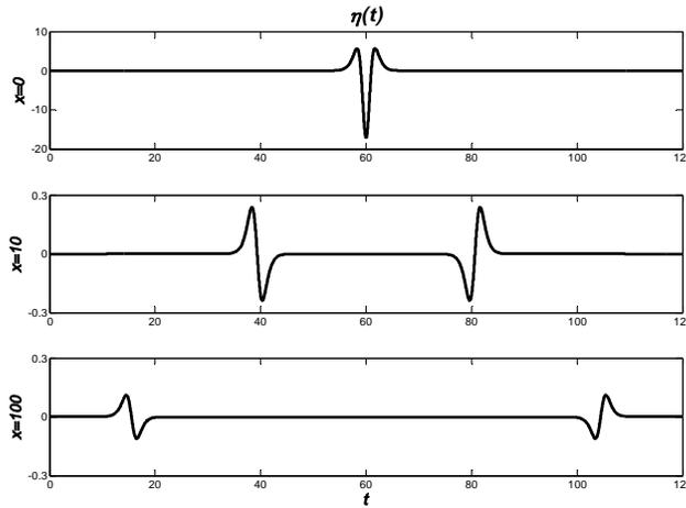
Fig. 1.4.1. Time series of the water surface of the wave system generated from the initial disturbance given by Eq. (1.3.12) at the shoreline and at two offshore points
