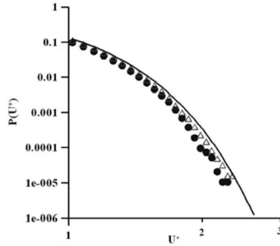
Fig. 3.4.2. Distribution functions of maximum velocities for incident wave (triangles) and shoreline displacement (circles) with the incident wave spectrum width  $l = 0.7$ . The solid line corresponds to the Rayleigh distribution
