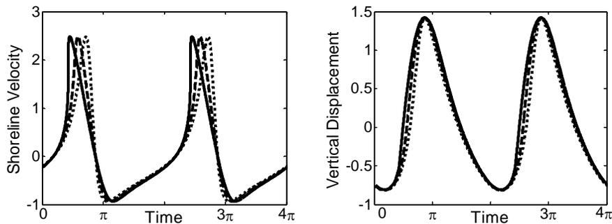
Fig. 2.5.4. Velocity and vertical displacement of the moving shoreline for a nonlinear deformed wave ( $s/s_0 = 2$ ) in non-dimensional variables; the breaking parameter  $Br = 0$  (dotted line),  $Br = 0.5$  (dashed line) and  $Br = 1$  (solid line)
