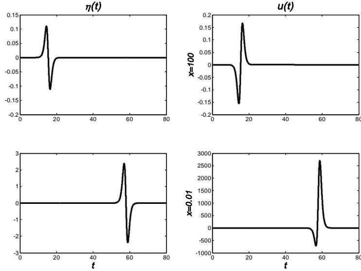
Fig. 1.2.1. The shape of a travelling wave (left) and the water flow (right) at various distances (m) from the shoreline. Time is given in seconds
