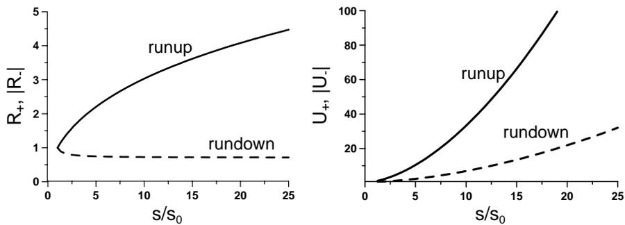
Fig. 2.5.3. Dependence of extreme runup ( $R_+$ ) and rundown ( $R_-$ ) heights and runup ( $U_+$ ) and rundown ( $U_-$ ) velocities (dimensionless variables) on the wave steepness
