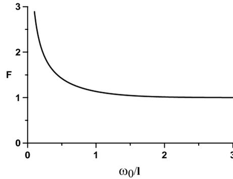
Fig. 3.4.3. Function of the influence of the incident wave spectrum width on the runup height of the wave
