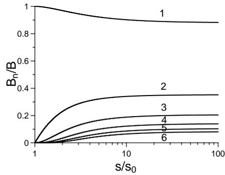
Fig. 2.5.2. Amplitudes of high harmonics versus face-slope steepness. Adapted from Paper II
