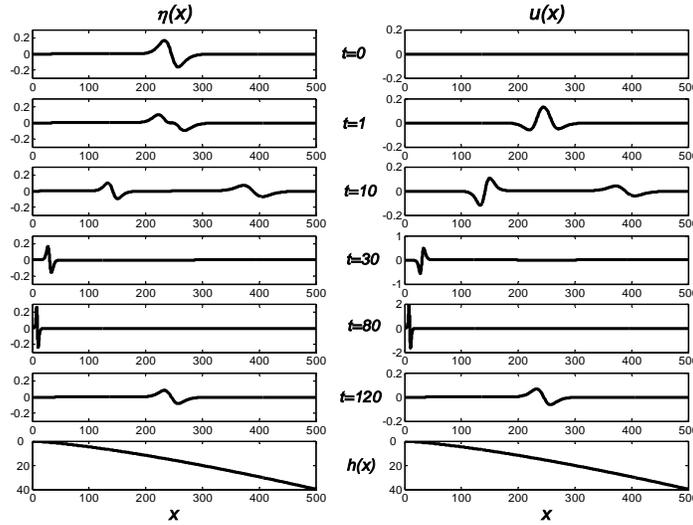
Fig. 1.3.1. Water displacement (left) and velocity (right) for initial disturbance (1.3.11). The bottom profile is shown at the bottom
