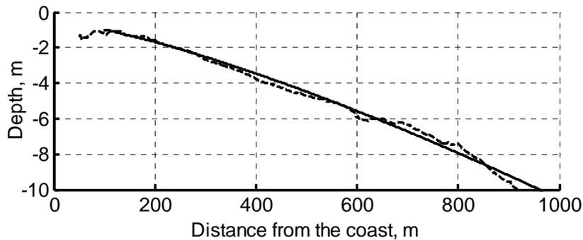
Fig. 1. The bottom profile measured at Pirita Beach, Estonia (dashed line) and its approximation with a power law with  $d = 4/3$  (solid line). Modified from Soomere et al. (2007)
