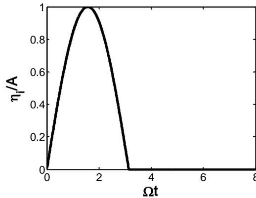
Fig. 1.5.2. Relative water surface elevation in the incident wave described by Eq. (1.5.8)
