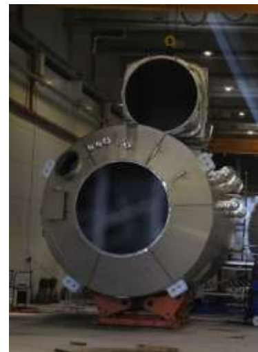
Scrubber; weight 16.6t; length 9.8m; diameter 3.8m
