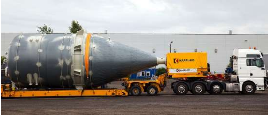
Reactor Dump Tank; weight 82.5 t; length 14.6m; diameter 4.5m; Finland
