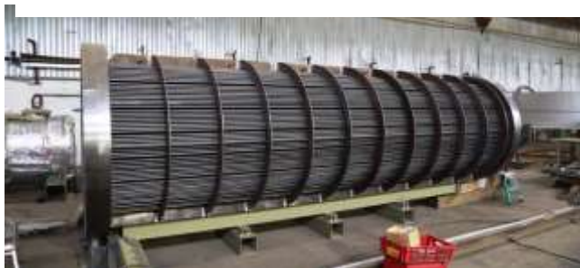
Heat exchanger; weight 23.1t; length 6.1m; diameter 1.8m
