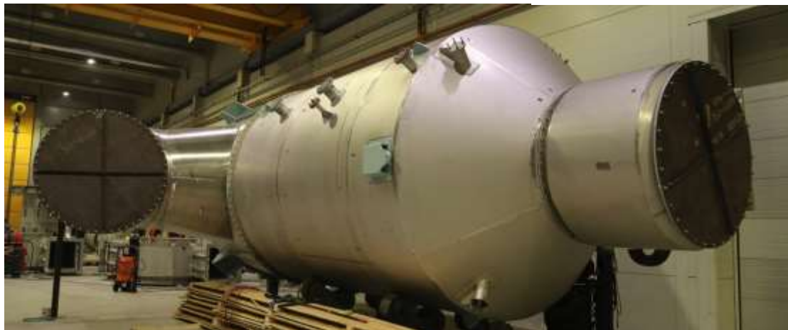
Scrubber; weight 10.8t; length 10.4m; diameter 3.5m
