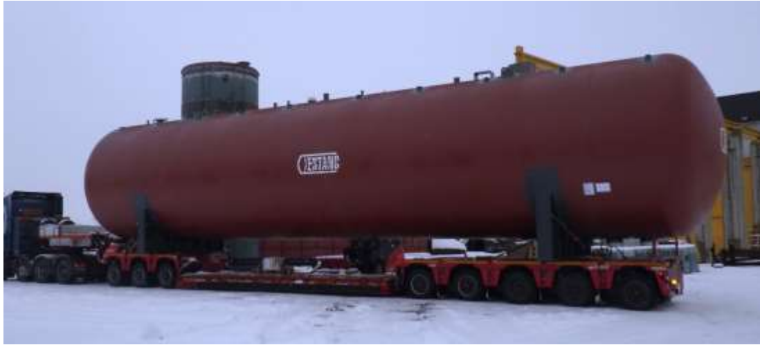
Feed water tank weight 76.5t; length 21.5m; diameter 4.5m; Finland
