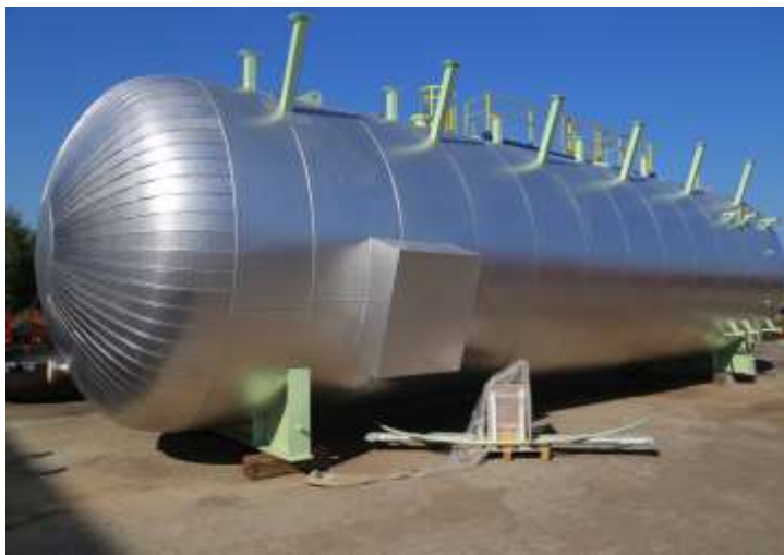
Feed water tank insulated; weight 22.5t; length 13m; diameter 3.3m
