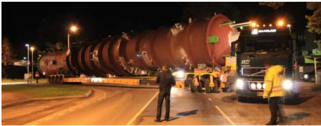
Condensing tower; weight 82t; length 33.6m; diameter 4.3m; Estonia
