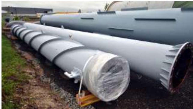
Chimney; weight 5.4t; length 27m; diameter 1m
