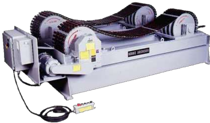
Figure 4.11 Sling type rotator Koike Trac-Tred T4 [15]
