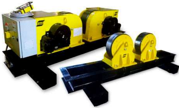
Figure 4.5 Conventional adjustable rotator ESAB CD-30 [11]
