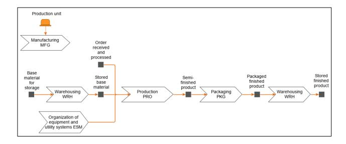
Figure 4. Manufacturing process of Vipis OÜ. Source: Midri (2019) author's compilation
