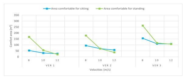
Figure 26.Comfort area size improved by Operable shelter in different comfort conditions
