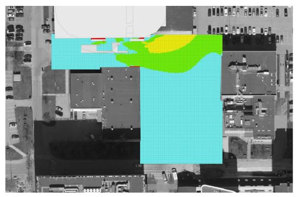
Figure 33. Wind comfort map for designed layout in Health Centre area
