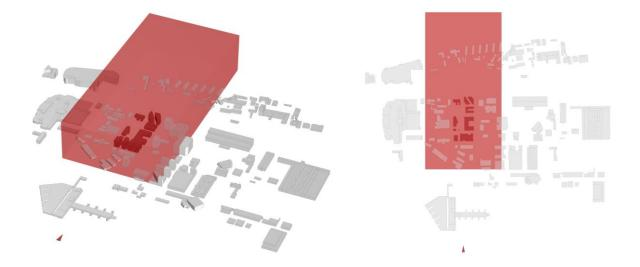
*Figure* 13. Rectangular wind tunnel for Lõõtsa park, red building are considered into simulation
