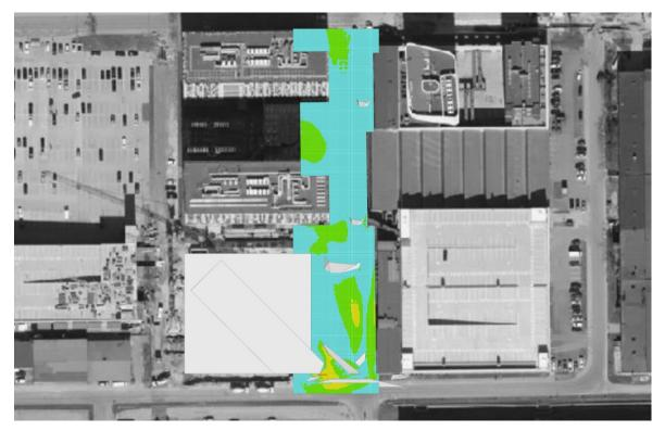
Figure 36. Wind comfort map for designed layout in Sepise street
