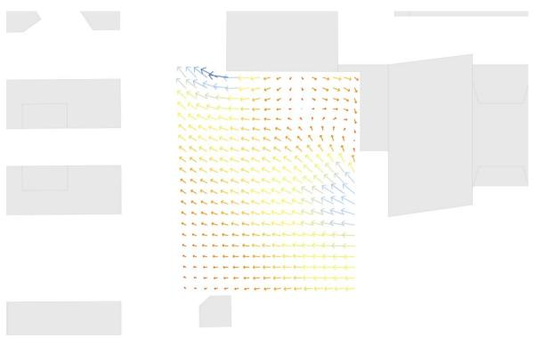
Figure 16.Wind flow and velocity plot in Viktor Palmi square 180°
