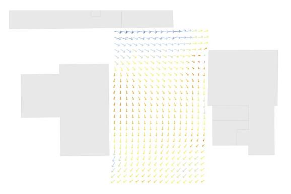
Figure 17. Wind flow and velocity plot in Health Centre park 202.5°
