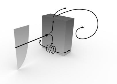
Figure 2. A schematic representation of wind flow around a single wide high-rise rectangular building
