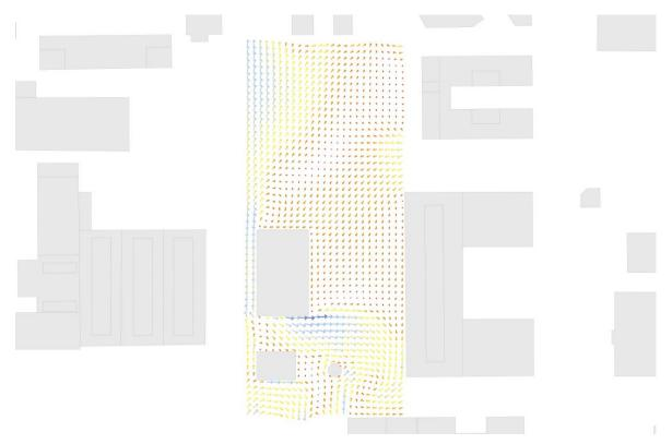
Figure 15. Wind flow and velocity plot in Lõõtsa park 180°
