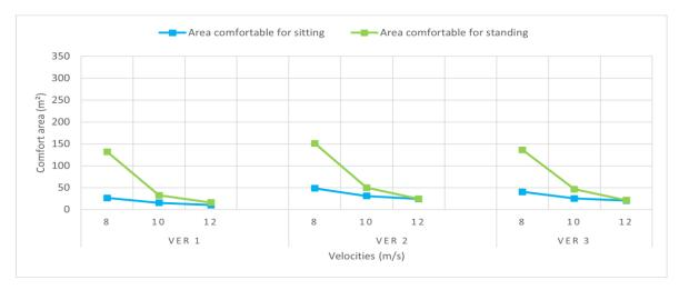
Figure 27.Comfort area size improved by Textile Wall shelter in different comfort conditions
