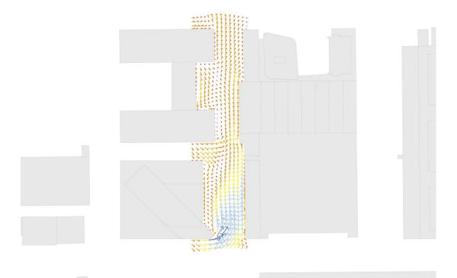
Figure 18. Wind flow and velocity plot in Sepise pedestrian street 180°
