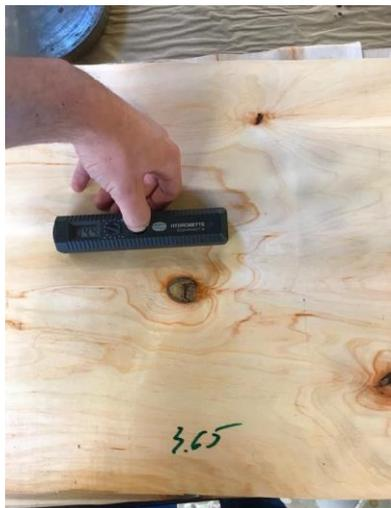
Figure 2.10 Dried veneer sheet with moisture content 4.4%
