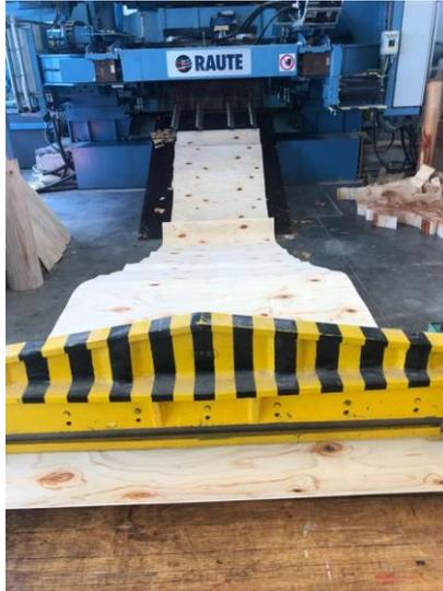
Figure 2.7 Guillotine for veneer cutting
