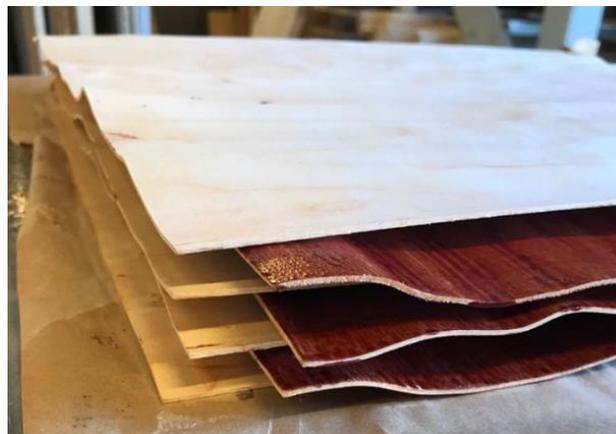
Figure 2.13 Glued veneer sheets before hot pressing process
