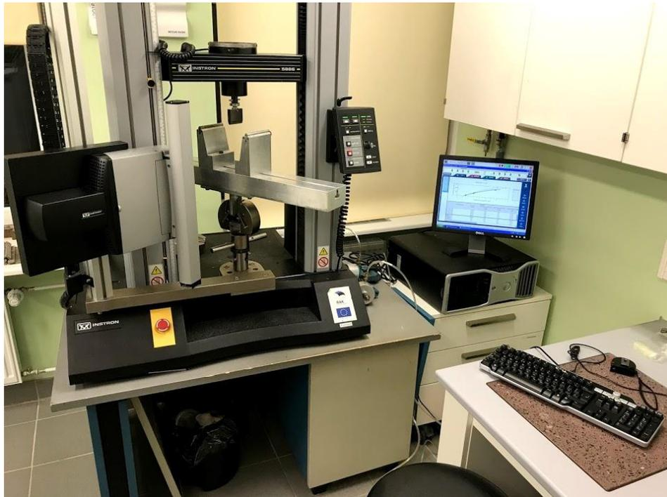
Figure 2.15 Instron 5866 apparatus for EN 310:2002 test at Tallinn University of Technology
