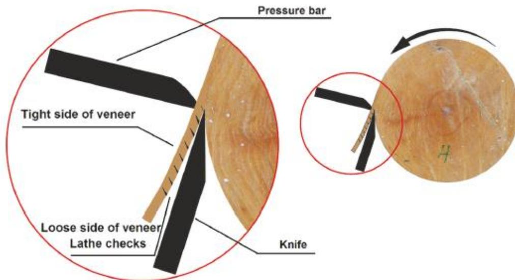
Figure 2.4 Tight and loose side explanation in peeling process [15]
