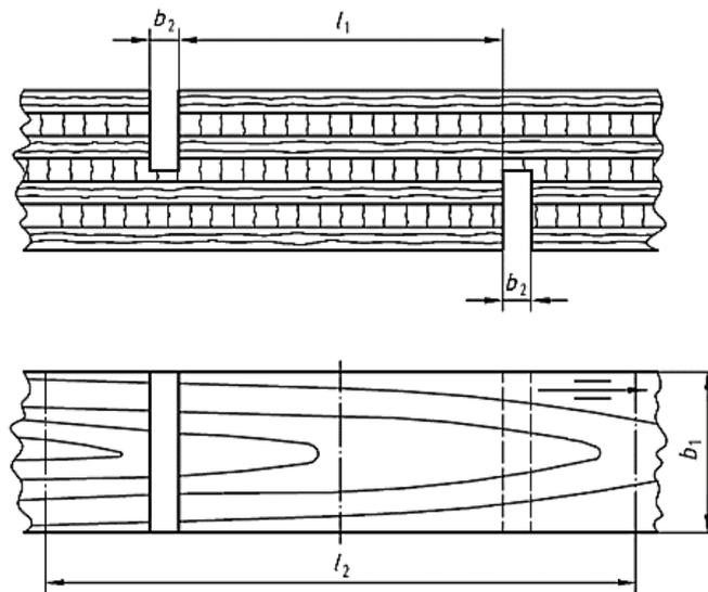
Figure 2.16 Test specimen example of 7-layers plywood [26]
