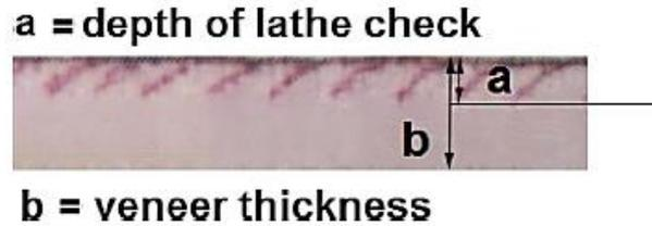
Figure 1.3 Overview of veneer lathe check depth (LCD) measurement [14]
