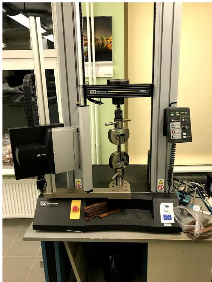
Figure 2.17 Instron 5866 apparatus for EN314-1:2005 test at Tallinn University of Technology
