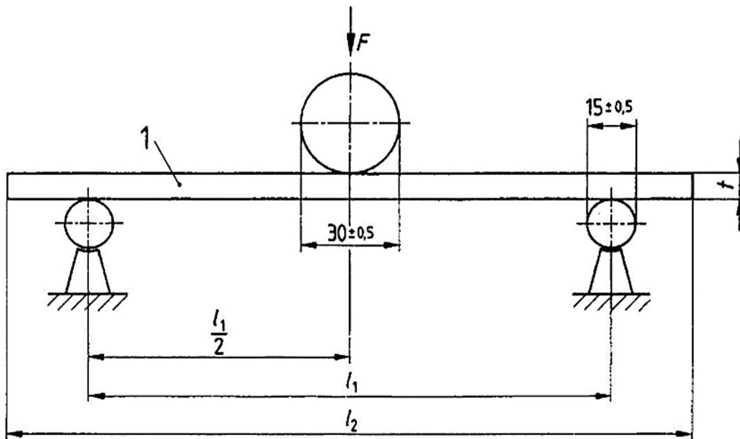
Figure 2.14 Testing apparatus according to the standard [24]
