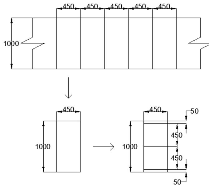
Figure 2.6 Veneer cutting process
