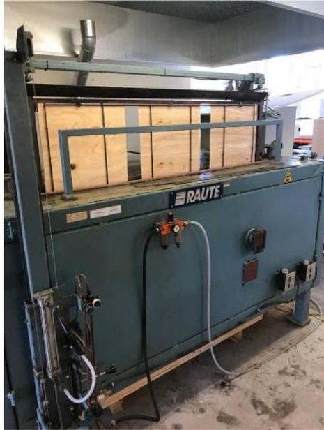
Figure 2.8 Veneer drying machine in TalTech Laboratory of Wood Technology
