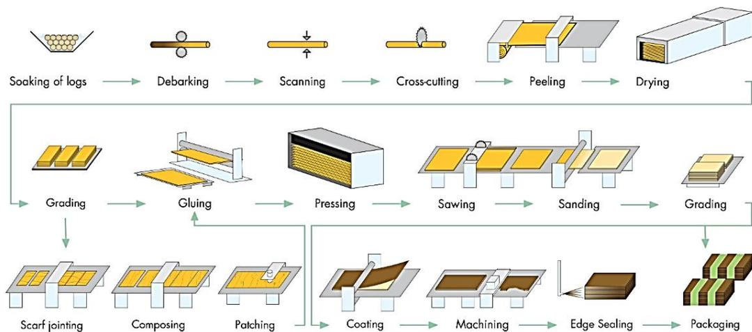
Figure 1.2 Plywood Production process [9]
