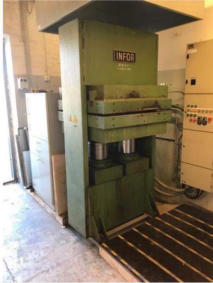
Figure 2.11 Hot press machine from Infor manufacturer
