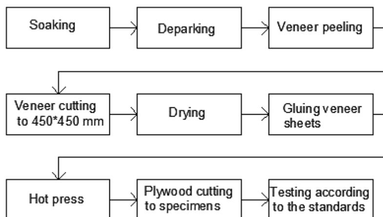
Figure 2.1 Plywood manufacturing processes in this study
