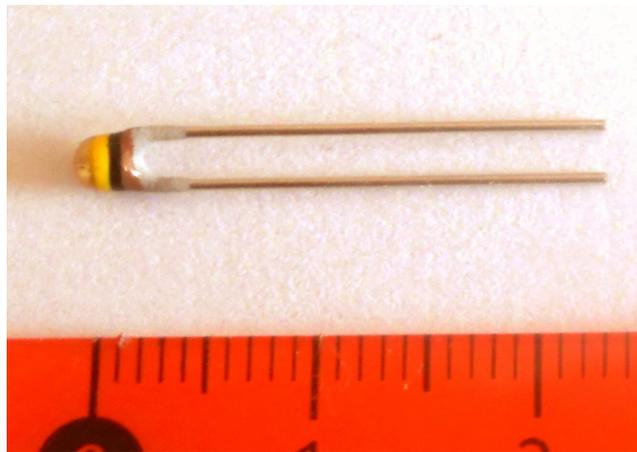
**Figure 1.** A photo of a typical NTC thermistor.
