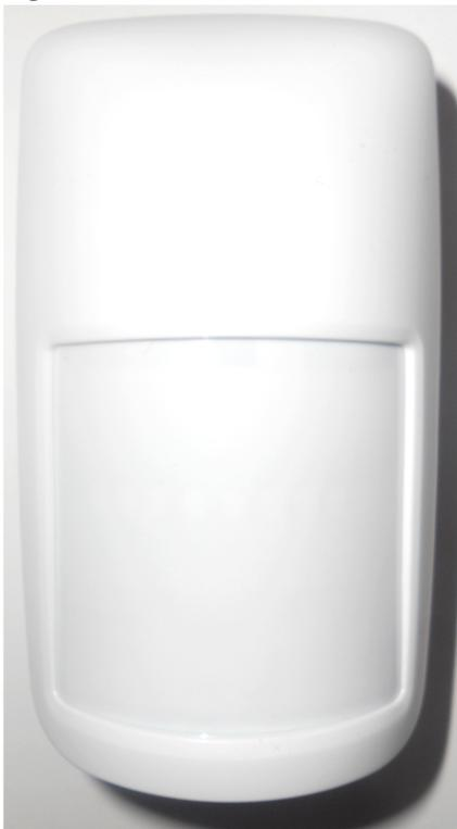
**Figure 2.** the outer view of the PIR
