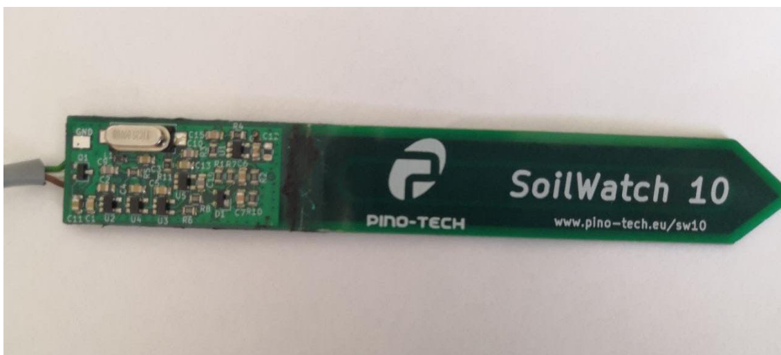
Figure 11: Pino-Tech SoilWatch 10 circuit
