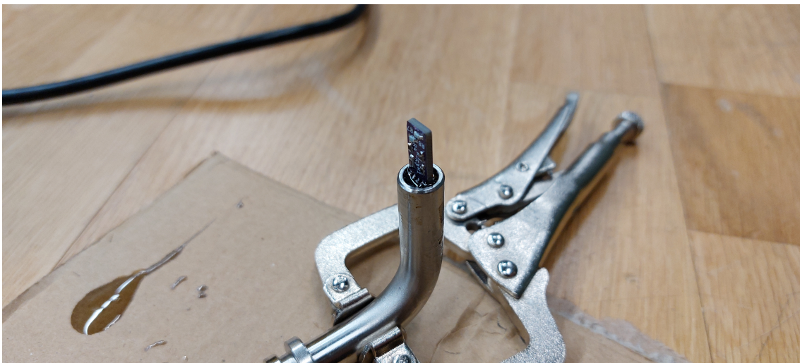
Figure 13. Pipe with the epoxied new sensor.
