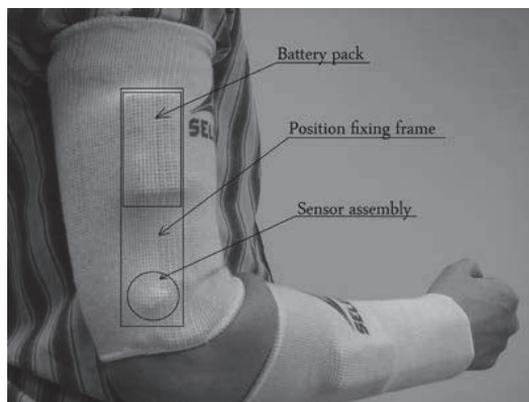
Figure 1. Wearing wireless MEMS sensors
