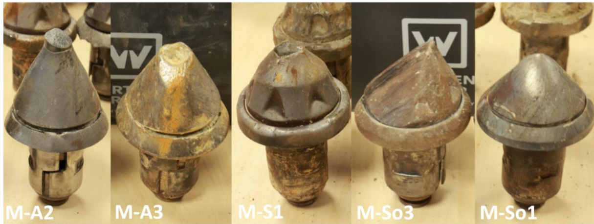
Figure 25. Different pick wear patterns observed in the discarded picks
