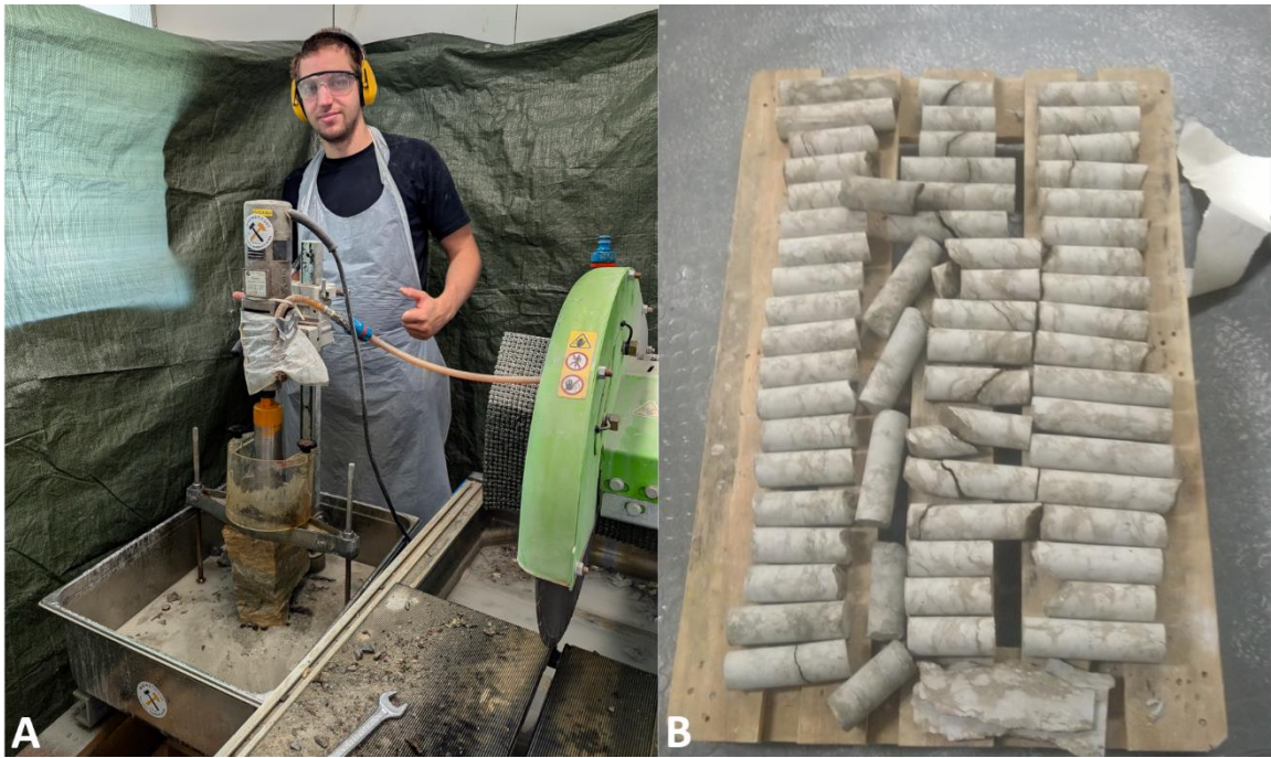
Figure 11. Sample preparation at Särghau. A – diamond drill used for coring of rocks; B – raw cores drilled from rock (photos by Reet Männik)
