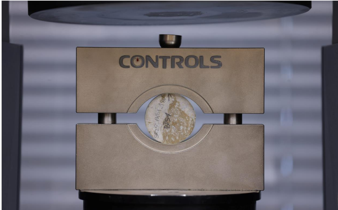
Figure 15. Setup for BTS tests (author's photo)
