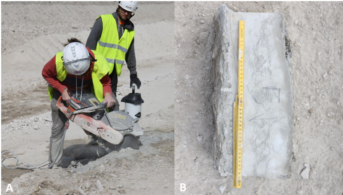
Figure 9. Sampling at the Põhja-Kiviõli mine. A – Limestone blocks being cut for sampling by Bruno Grafe, assisted by Sander Kanter. B – a block cut from layer 5. (photos by the author)
