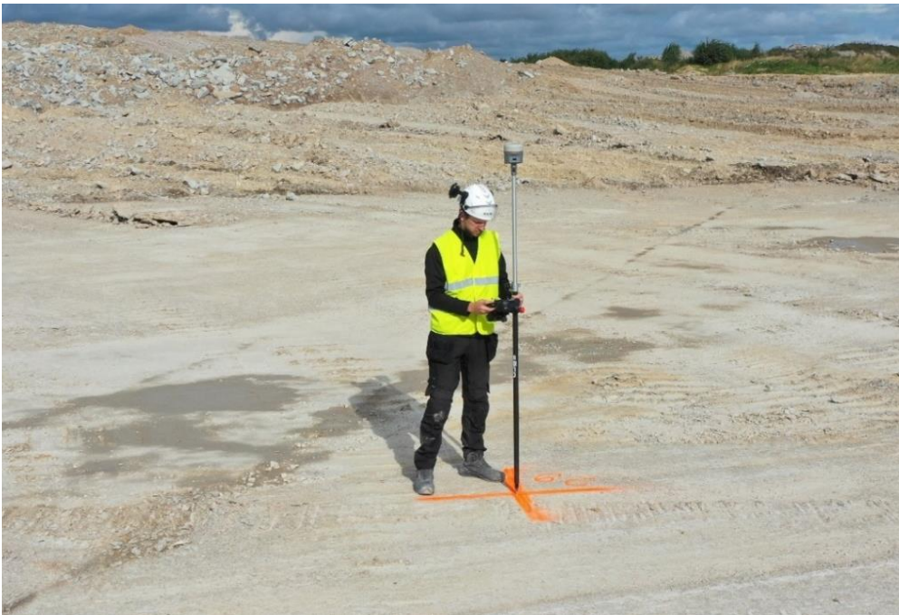
Figure 7. Measuring the coordinates of GCP-29 using the Trimble R10 (author's photo)
