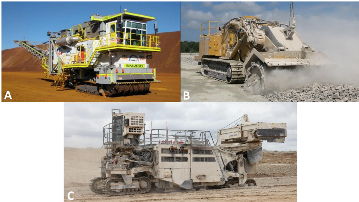
Figure 2. Surface miners with different drum configurations. A – front cutting drum (Takraf TSM 300) (Directindustry, 2026); B – rear cutting drum (Vermeer T1255) (Department of Mining, 2012); C – central cutting drum (Wirtgen 280 SMi) (author’s photo, 2025)
