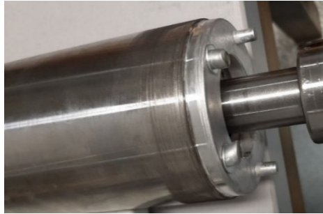
Figure 8. Rotor wear caused by centrifugal forces.
