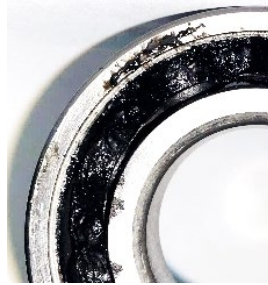
Figure 37. Lubricant darkening due to discharges.
