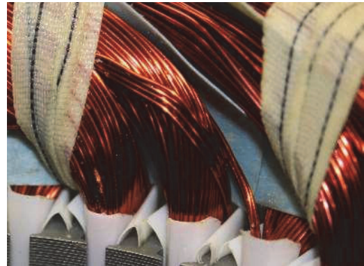
Fig. 2. Insulation damage and improper winding placement in Motor 2.
