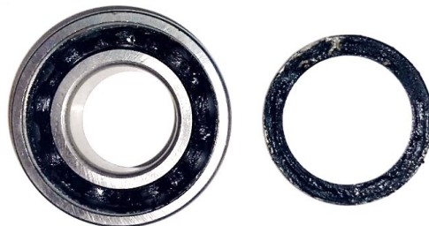
Figure 5. Improper lubrication of bearing. (previously published in article 1)
