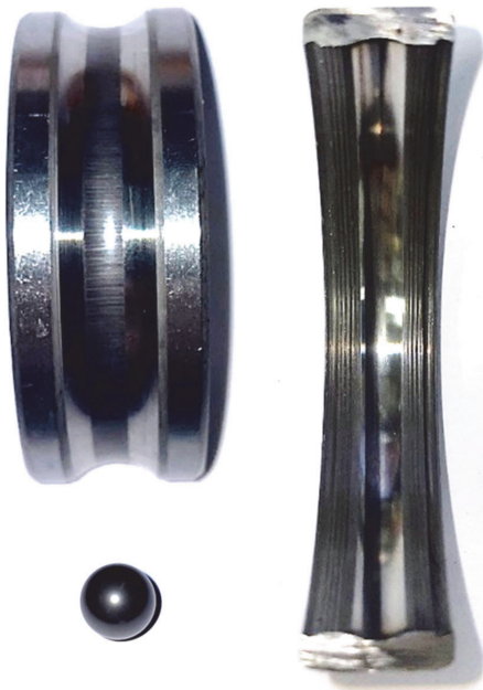
Fig. 5 DE bearing at 500 r/min and 10 A
