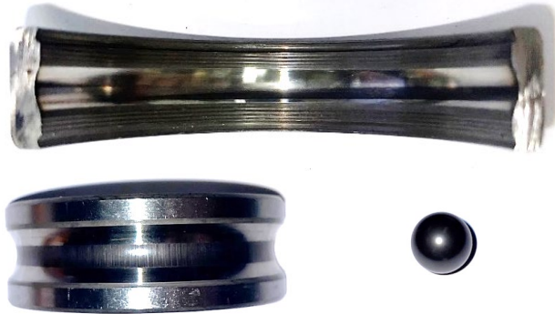
Figure 39. Bearing with fluting used in experiments. (previously published in article VI)
