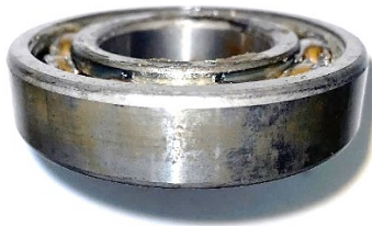
Figure 4. An example of corroded bearing. (previously published in article 1)
