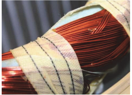
Fig. 7. Insulation damage in Motor 6.
