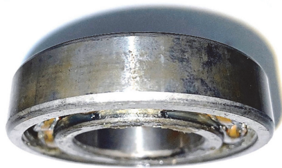
Figure 3. Corroded surface of a rolling bearing.
