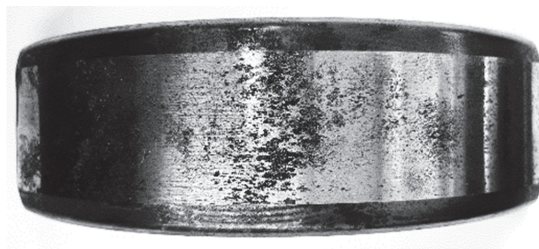
Figure 2. Material fatigue of a rolling bearing.
