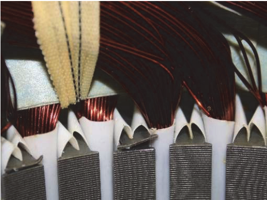
Fig. 5. The curvature of the lamination stacks in Motor 4.
