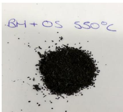
Figure 41. Char obtained with Biomass and Oil Shale at 550°C
