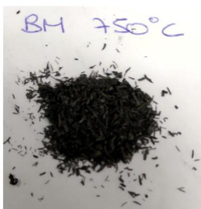
Figure 36. Char obtained with Biomass at 750°C
