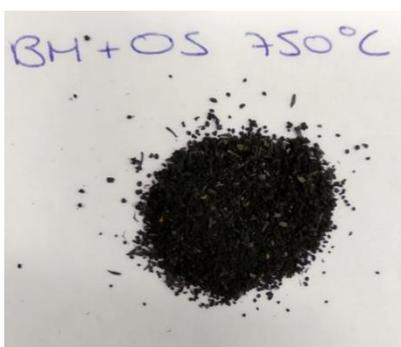
Figure 42. Char obtained with Biomass and Oil Shale at 750°C
