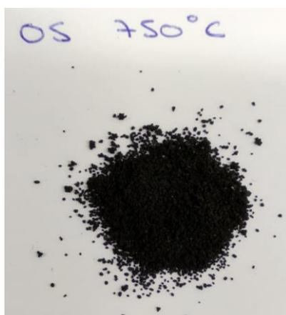
Figure 39. Char obtained with Oil Shale at 750°C
