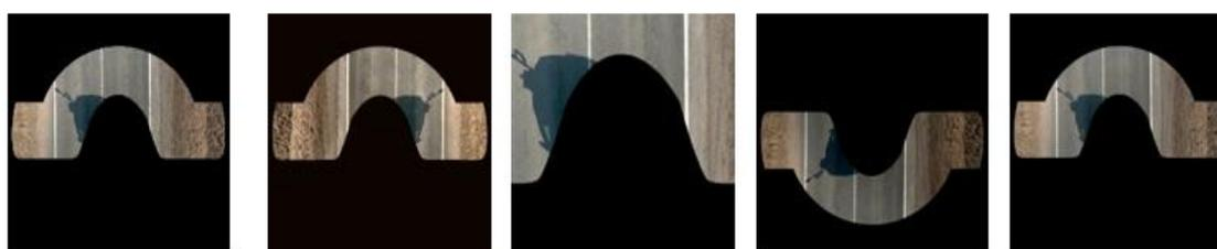
Figure 3.4 Example of orthoframe augmentation. The first image on the left is the original image, followed by random brightness, center crop, vertical flipping, and random contrast transformations, respectively.
