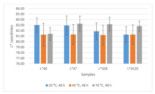
Figure 3.10 L\* (lightness) coordinates for dried birch veneer samples from logs soaked for 20  $^{\circ}$ C, 40  $^{\circ}$ C, and 70  $^{\circ}$ C at different intervals (0, 7, 28, and 120) days after drying
