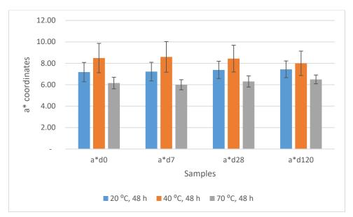
Figure 3.9 a\* (red) coordinates for dried birch veneer samples from logs soaked for 20  $^{\circ}$ C, 40  $^{\circ}$ C, and 70  $^{\circ}$ C at different intervals (0, 7, 28, and 120) days after drying
