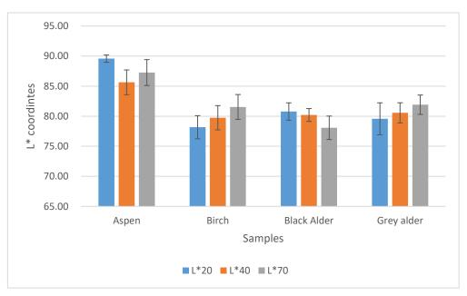
Figure 3.1 L\* (lightness) coordinates of aspen, birch, black and grey alder for 24 h at different soaking temperature
