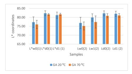
Figure 3.19 Colour coordinate L\* values for 1mm grey alder samples with different drying after peeling (1) first set dried immediately after peeling and (2) dried after 24 h. Where Lw0 is wet veneer, Lw1 is wet veneer after 24 h, Ld0 is freshly dried veneer, and Ld1 is dried veneer after 7 days
