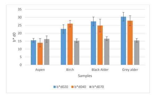
Figure 3.6 b\* (yellow) coordinates of aspen, birch, black and grey alder for 24 h at different soaking temperature. Where b\*d020, b\*d040, and b\*d0 is freshly dried veneer samples peeled at 20, 40, and 70  $^{\circ}$ C, respectively
