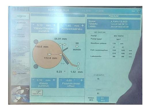
Figure 2.2 Machinery setting for peeling 1.5mm thick veneer mat
