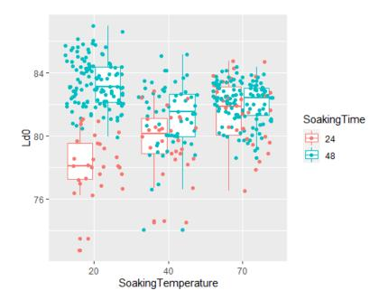
Figure 3.12 L\* (lightness) coordinates of the birch samples with 24 h and 48 h soaking duration.
