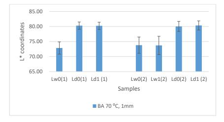
Figure 3.20 Colour coordinate L\* values for 1mm black alder samples with different drying time after peeling (1) first set dried immediatetely after peeling and (2) dried after 24 hours. Where Lw0 is wet veneer, Lw1 is wet veneer after 24 h, Ld0 is freshly dried veneer, and Ld1 is dried veneer after 7 days
