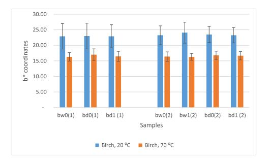
Figure 3.17 Colour coordinate b\* values for 1mm birch samples with different drying time after peeling (1) first set dried immediately after peeling and (2) dried after 24 h. Where bw0 is wet veneer, bw1 is wet veneer after 24 h, bd0 is freshly dried veneer, and bd1 is dried veneer after 7 days
