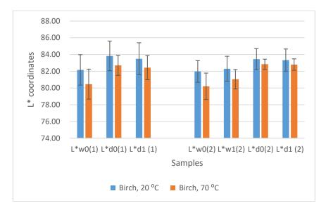
Figure 3.15 Colour coordinate L\* values for 1mm birch samples with different drying time after peeling (1) first set dried immediately after peeling and (2) dried after 24 h. Where Lw0 is wet veneer, Lw1 is wet veneer after 24 h, Ld0 is freshly dried veneer, and Ld1 is dried veneer after 7 days
