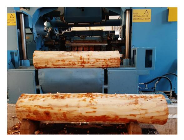
Figure 2.1 Debarked logs fed into the rotary veneer peeling lathe
