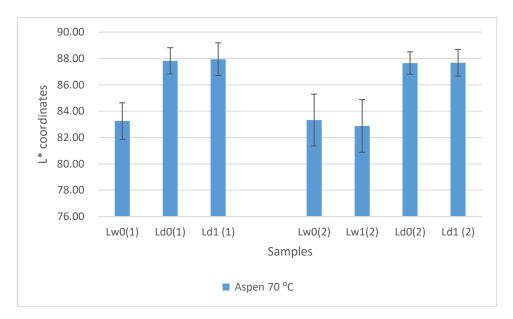
Figure 3.18 Colour coordinate L\* values for 1mm aspen samples with different drying time after peeling (1) first set dried immediately after peeling and (2) dried after 24 h. Where Lw0 is wet veneer, Lw1 is wet veneer after 24 h, Ld0 is freshly dried veneer, and Ld1 is dried veneer after 7 days
