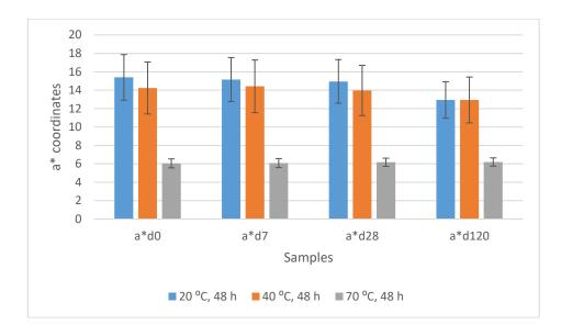
Figure 3.11 a\* (red) coordinates for dried grey veneer samples from logs soaked for 20 °C, 40 °C, and 70 °C at different intervals (0, 7, 28, and 120) days after drying
