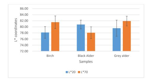
Figure 3.5. Differences in L\* (lightness) coordinates of birch veneer prepared at 20 °C and 70 °C soaking temperature and at 48 h soaking duration
