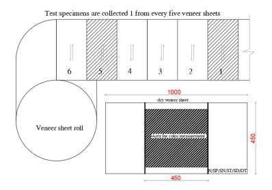
Figure 2.6 Specimen sampling plan for colour measurement. The number of veneer sheet samples and colour measurements taken varies across the log samples.
