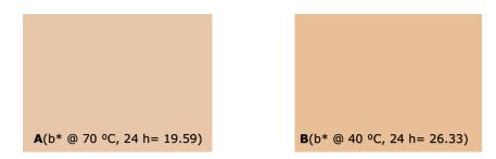
Figure 3.4 The colour tone of veneer soaked at 40 °C and 70 °C for 24h
