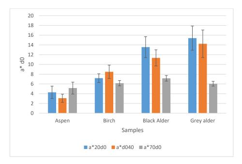
Figure 3.7 a\* (red) coordinates of aspen, birch, black and grey alder for 24 h at different soaking temperature, where a\*d020, a\*d040, and a\*d0 is freshly dried veneer samples peeled at 20, 40, and 70  $^{\circ}$ C, respectively
