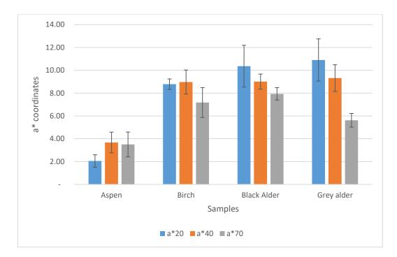
Figure 3.2 a\* (red) coordinates of aspen, birch, black and grey alder for 24 h at different soaking temperature
