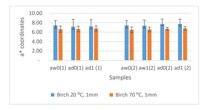
Figure 3.16 Colour coordinate a\* values for 1mm birch samples with different drying time after peeling (1) first set dried immediately after peeling and (2) dried after 24 h. Where aw0 is wet veneer, aw1 is wet veneer after 24 h, ad0 is freshly dried veneer, and ad1 is dried veneer after 7 days
