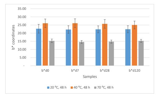
Figure 3.8 b\* (yellow) coordinates dried birch veneer samples from logs soaked for 20 C, 40 C, and 70 C at different intervals (0, 7, 28, and 120) days after drying.
