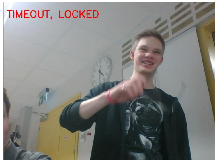
Figure 4.6. The prototype system recognizing an unknown individual and forbidding entry in the timeout state.
