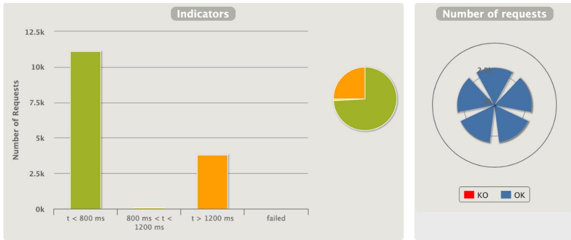
Figure 38. SPRUT microservice load testing results with 1000 users and 5000 requests
