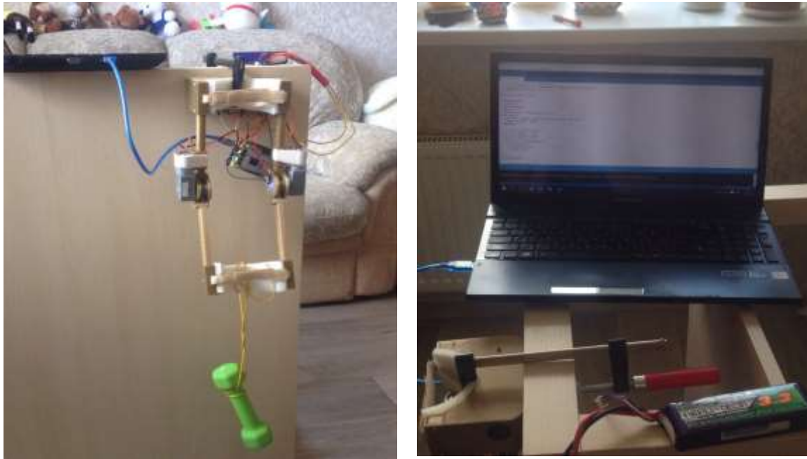
Figure 5.9 Testing installation with 1.75 kg load
