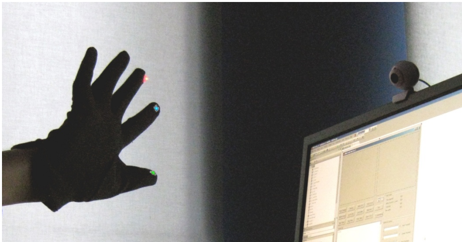
Figure 4.3 Glove with LED's and the camera
