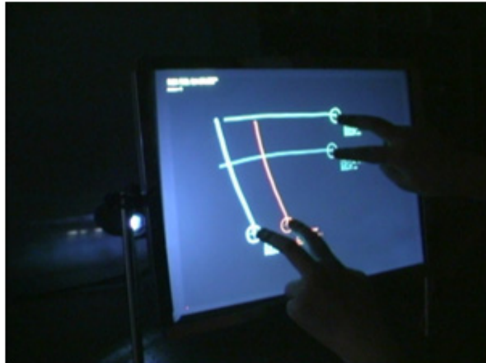
Figure 2.8 Multi-touch screen implementation, using FTIR technology (picture from cs.nyu.edu/~jhan/ )
