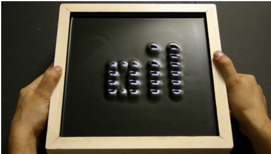
Figure 2.5 SnOil – a tactile surface based on ferro fluid (picture from www.freymartin.de )
