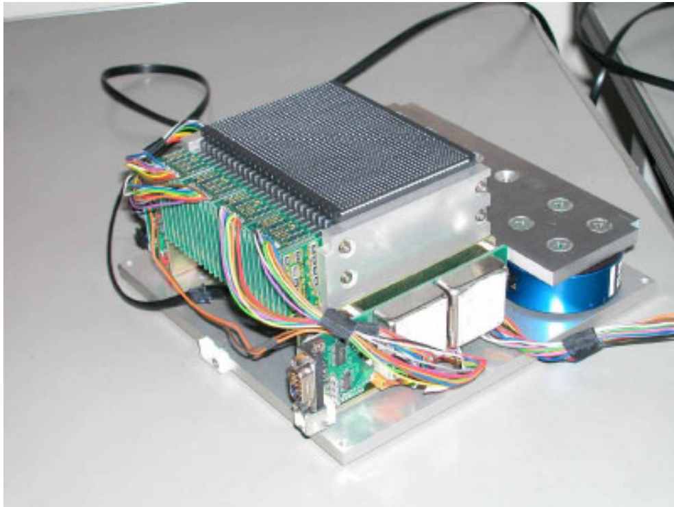
Figure 3.3 The prototype tactile display (picture from www.aist.go.jp )
