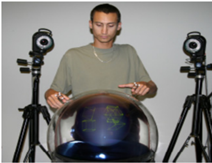
Figure 2.15 Volumetric display with camera based finger tracking system (picture from www.acm.org )
