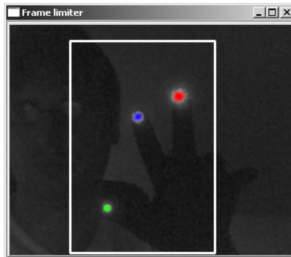
Figure 4.4 Trackframe painted around LED's on captured image
