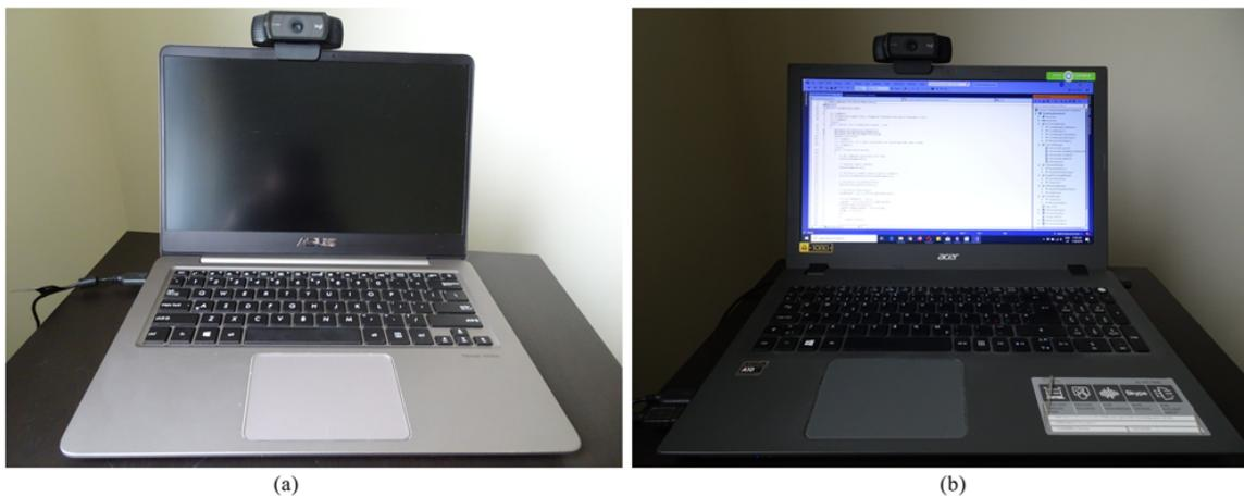
Figure 6.1: Hardware setup (Logitech C920 webcam mounted to two different laptops using universal clip mount support)
