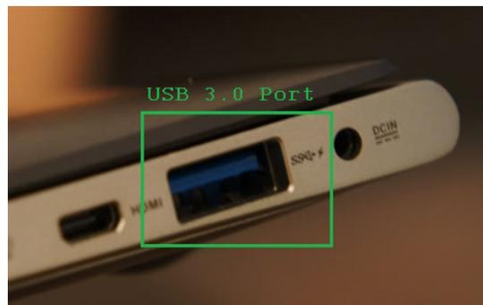
Figure 6.2: USB 3.0 port in laptop where webcam should be connected
