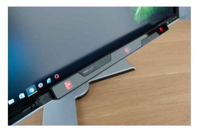
Figure 15 Mounting of the EyeX controller (Source: http://www.pcworld.com/article/3014523/peripherals/tobii-eyex-review-the-eye-mouse-is-magical-but-just-not-for-everyone.html)
