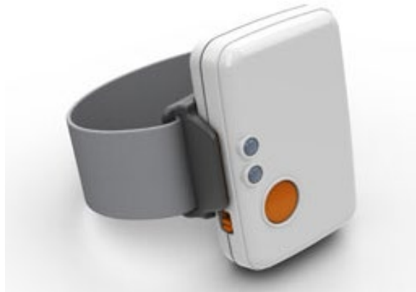
Figure 3. Shimmer3 IMU, which was used for measuring and recording acceleration signals from the left wrist. Signals were recorded with a dynamic range of \pm 16 g and numeric resolution of 16-bit with the built-in accelerometer STMicroelectronics LSM303AHTR (Shimmer Research).
