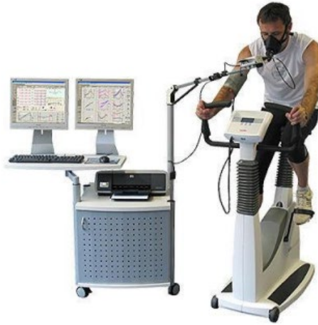
Figure 4. Carefusion Masterscreen CPX spirometry device. Alternative set-up with treadmill was used for indirect calorimetry measurements during “indoor test 2” and “indoor test 3”. MasterScreen CPX allows for breath-by-breath indirect calorimetry measurements using Weir equation by measuring oxygen consumption and carbon dioxide production (CareFusion).
