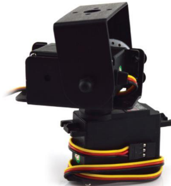
Joonis 4.2 Lynxmotion Pan and Tilt Kit / Aluminium [15]
