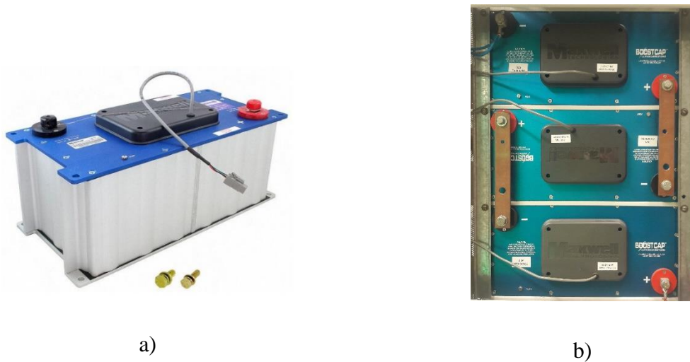
Figure 17 Supercapacitor module c [6] (a) and series connection of three modules in test bench (b).
