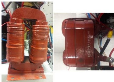
Figure 14 Inductor that was used in the converter.
