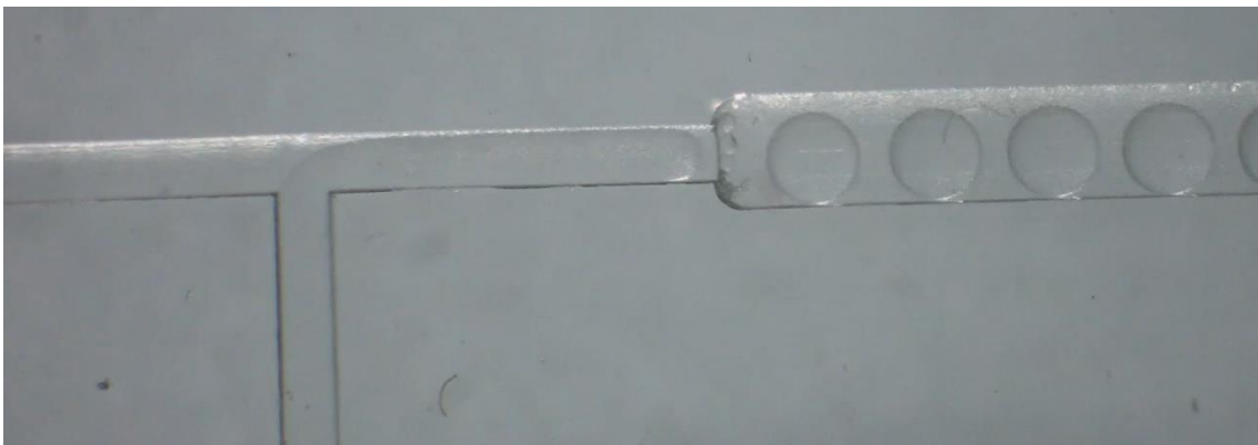
Figure 27. T-cross flow chip layout (droplets generated with reference KF technology syringe pumps)
