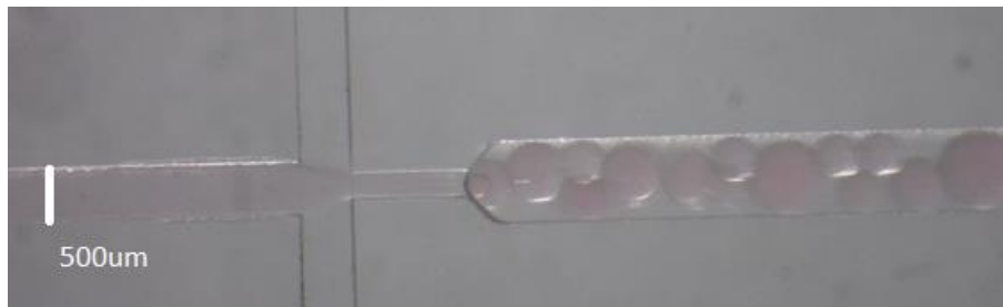
Figure 29. Generated droplets (two-phase emulsion) using the peristaltic pump developed in this thesis
