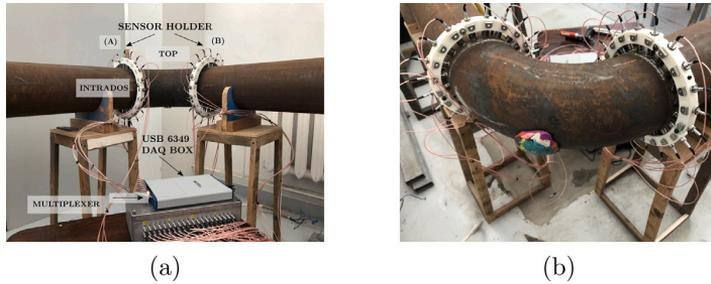
Fig. 13. Experimental setup: (a) measurement setup with transducer arrays A and B with 20 transducers each and an acquisition system; (b) pipe bend with an artificial defect composed of plasticine and located on the extrados position. The experimental pipe dimensions are the same as described in Section 2.4, with the only exception being the straight pipe dimension whose longitudes are 1 m each to avoid reflections with the edges.
