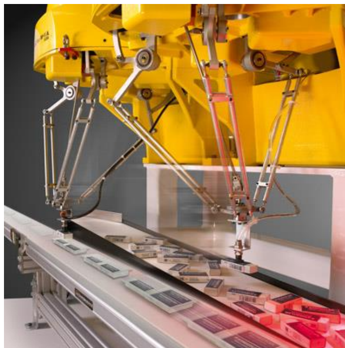
Figure 1.1 Fanuc Delta robots performing tasks in an assembly [3]
