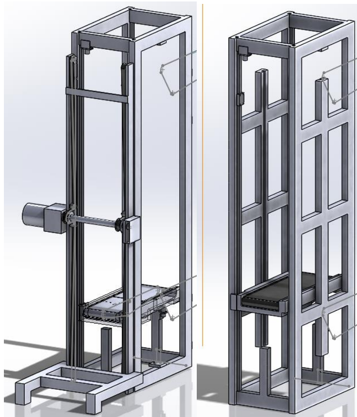
Figure 4.3 AC motor vertical lift (left) and DC stepper motor (right)
