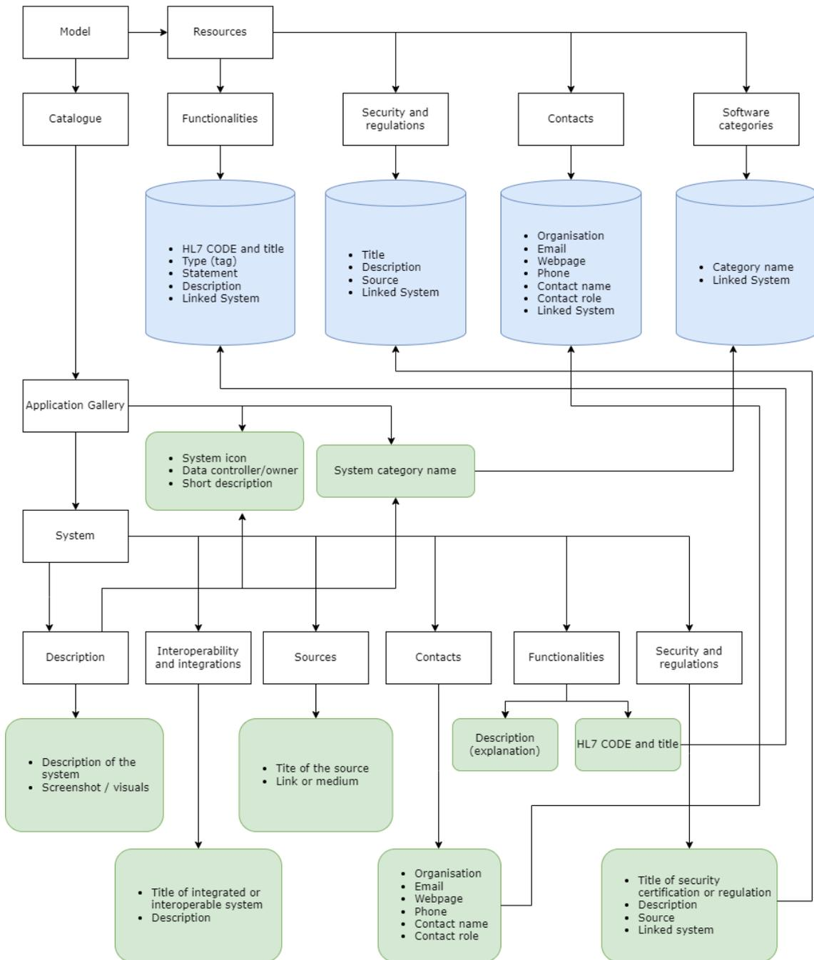
Figure 2. The basic architecture of e-health system mapping prototype. The architecture is based on the capabilities of the Notion platform. The blue cylinders refer to back-end data sets. White boxes are sections, green boxes are data, and the arrows show connections between sections.
