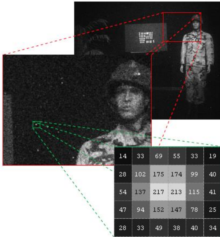
Figure 2-1: Example of scintillation noise from an intensified digital imager [4]
