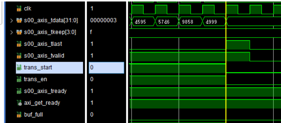
Figure 5-12: Simulation result of “AXI receiver” when receiving is going to finish
