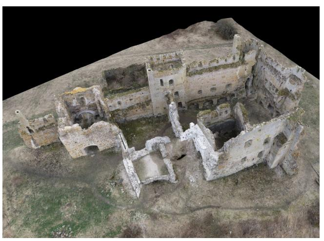
Illustration 28 The model of the Toolse castle done with photogammetry with dronedeploy software (by author)
