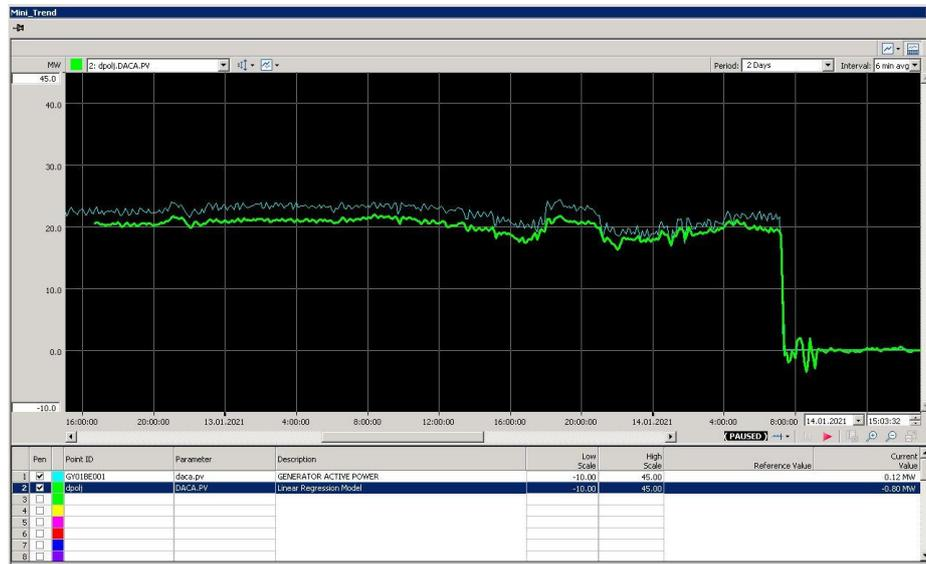
Figure 58. Comparative graphs of actual and predicted turbine load.
