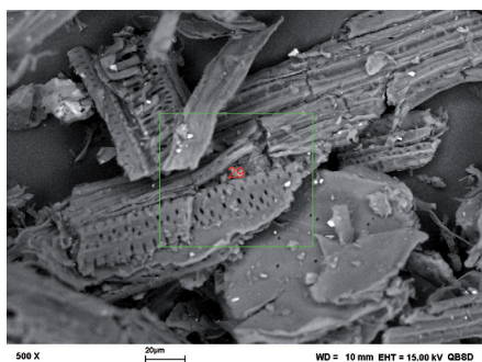
c) Different shape of particles with longitudinal cavities and network of holes
