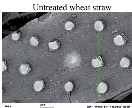
a) Oblong particle with holes and silicon bubbles
