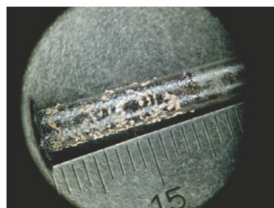
Figure 11. Sample of the gasification residue of PP800.
