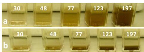
**Figure 2.** Effect of test medium composition on the agglomeration of CuO nanoparticles. Suspensions of nCuO in MQ water (a) and Osterhout's mineral medium (b) after 3 h at room temperature. The numbers refer to the nominal concentrations of nCuO (mg/L).
