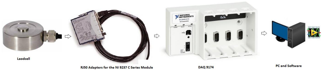
Figure 30. Load Cell data acquisition system
