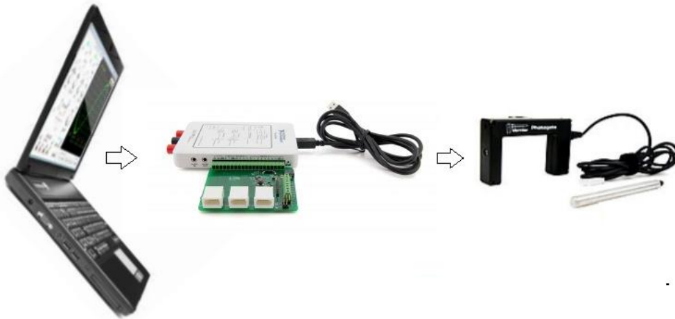
Figure 36. myDAQ connects the PC to Photogate sensor
