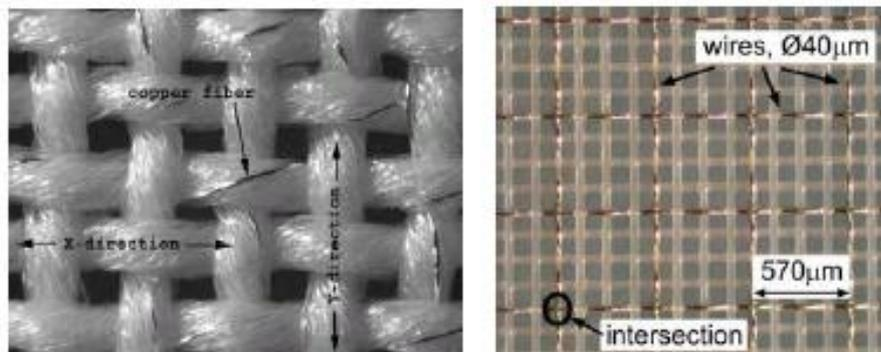
Figure 7. Conductive fabric from copper and polyester yarns [12].
