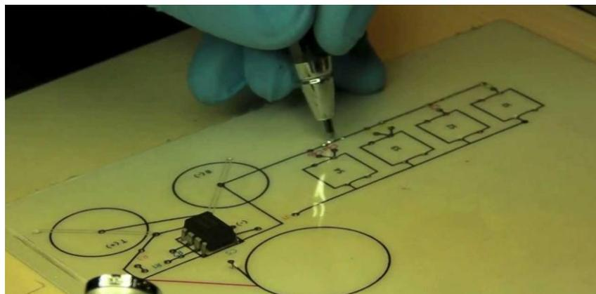
Figure 8. Drawing with conductive ink [12].
