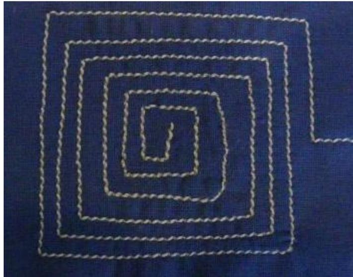
Figure 11. Textile antenna made from inox thread [12].
