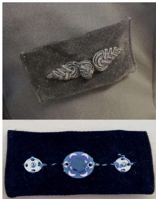
Figure 34. Buzzer on right chest piece.
