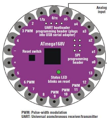
Figure 13. Diagram of the Lilypad microcontroller module [21].
