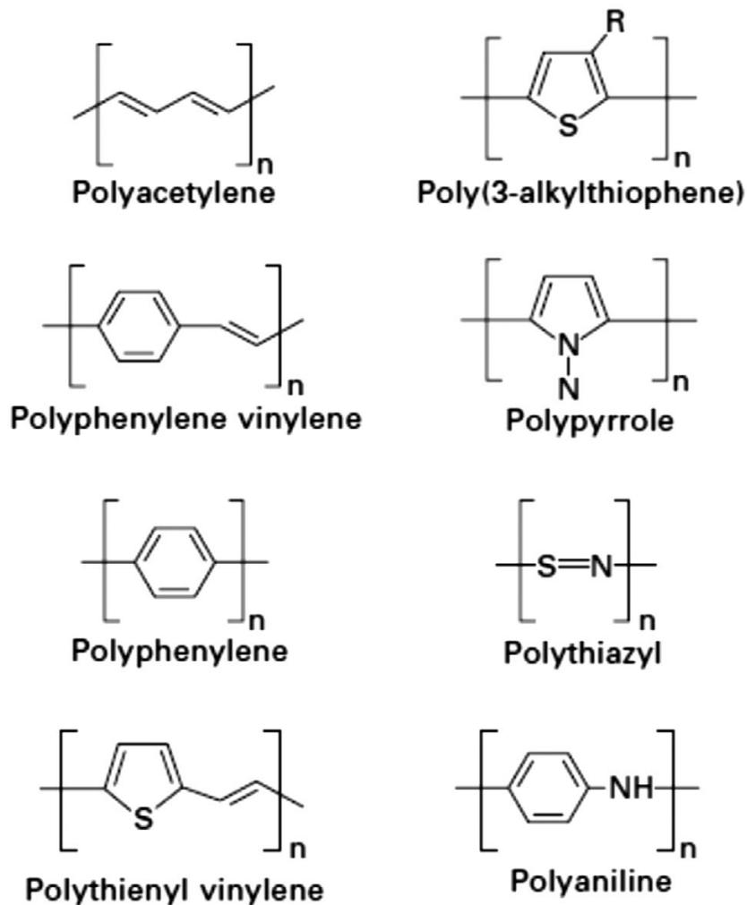
Figure 6. Chemical structure of more popular electrically conductive polymers [13].
