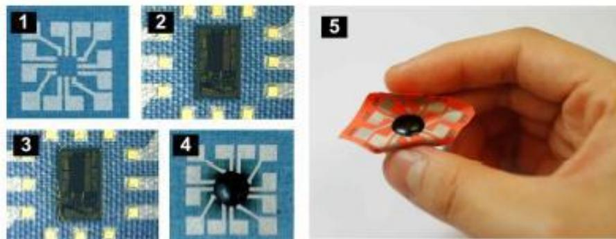
Figure 10. Single-layered P-FCB system manufacturing process [12].
